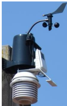
Figure 24. Weather station Wireless Vantage Pro 2 Station.
