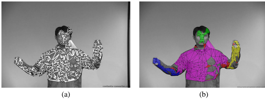
Figure 3.6: (a) Triangulated graph. (b) Result of grouping by irregular pyramid. Reprinted from [ 11] with permission from Elsevier.
