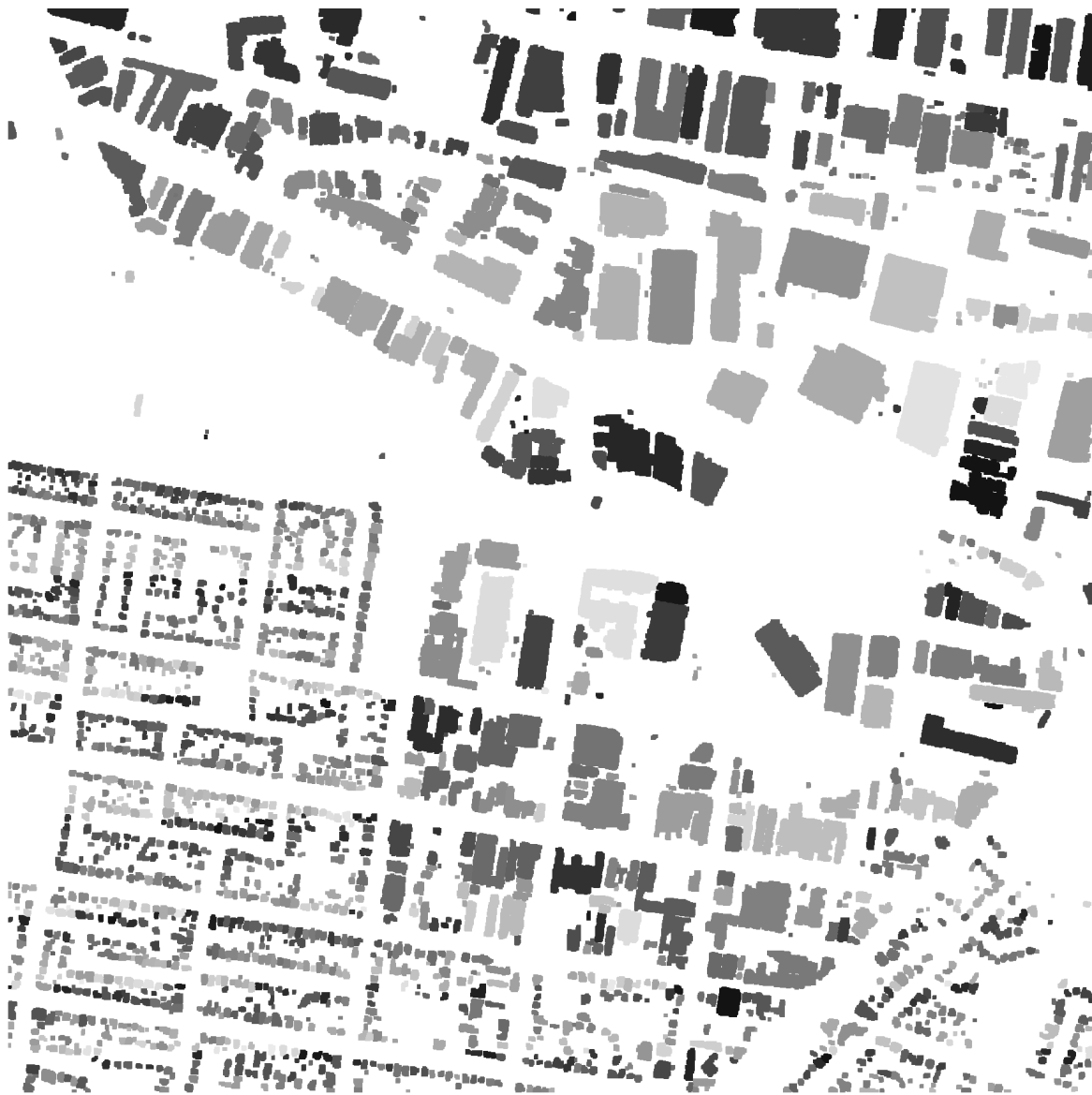
Figure 4.7: The final building label image after the second Dempster-Shafer classification and after growing the building regions by morphological closing.
