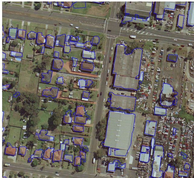
Figure 3.7: Boundary polygons super-imposed to the orthophoto.
