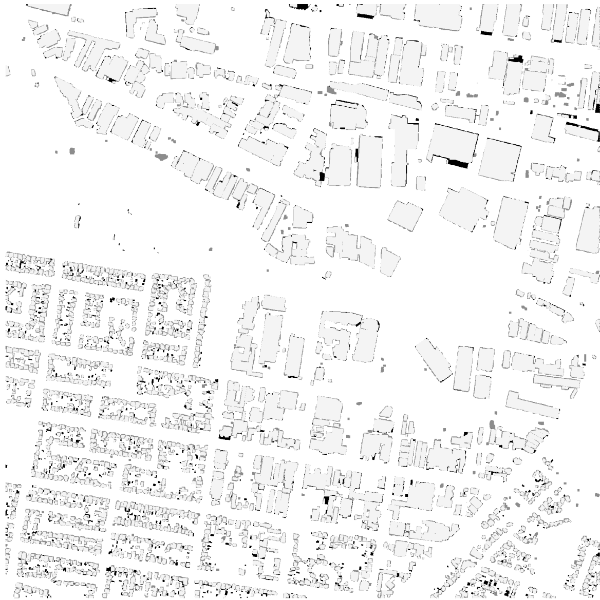
Figure 4.8: Evaluation of the results of building detection. Light grey: correct building pixels; medium grey: false positives; black: false negatives.
