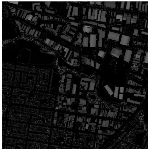
Figure 4.4: The normalised DSM used in Dempster-Shafer classification (black: low areas, white: high areas).
