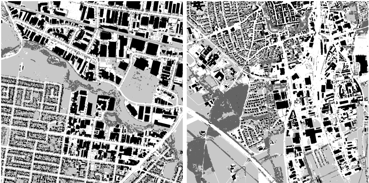
Figure 5.7: Results of the Dempster-Shafer classification after post-processing for Fairfield (left) and Memmingen (right). White: bare soil. Light grey: grass land. Dark grey: trees. Black: buildings.
