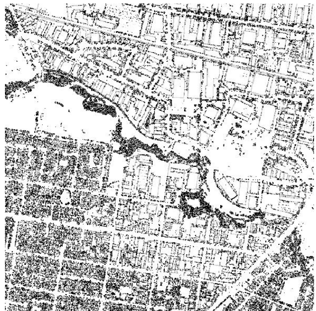
Figure 3.5: The classification results of polymorphic feature extraction. White: "homogeneous", light grey: "linear", black: "point-like".
