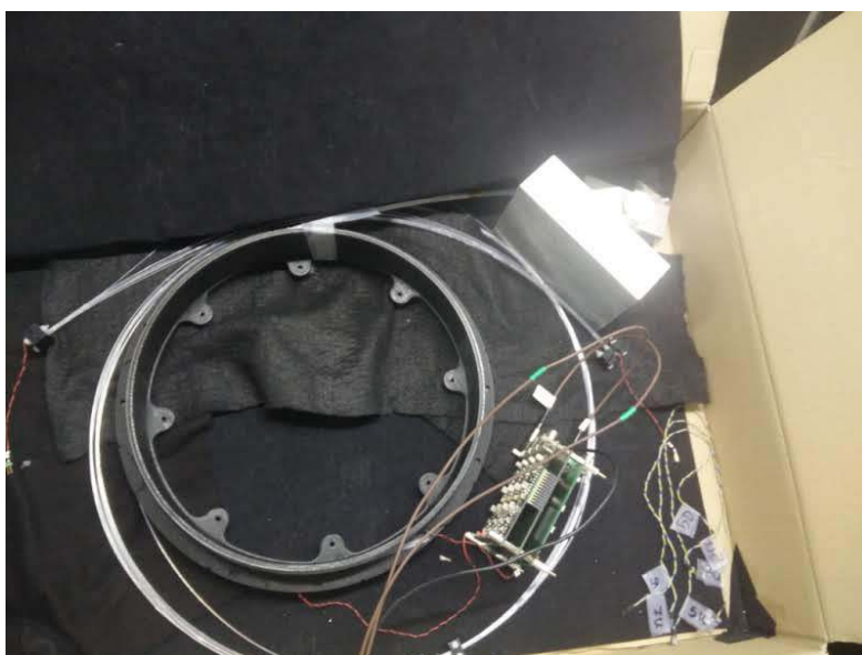
Figure 4.8.: Setup for the crosstalk measurements. A 3D printed model of the outer layer is used. The \text{Sr}_{90} source is shielded by an aluminium block.
