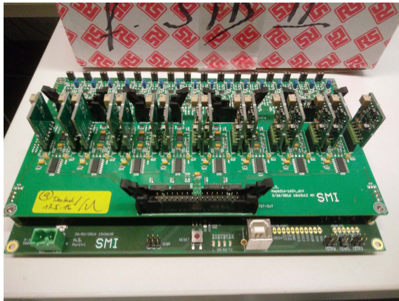
Figure 5.6.: The successor to the IFES board. On the upper end, the SIPMs are connected, the small pin-header connectors provide analogue output, the large connector digital ToT signals. On the lower level motherboard, the power connector is seen on the left, and right to the middle the USB connector
