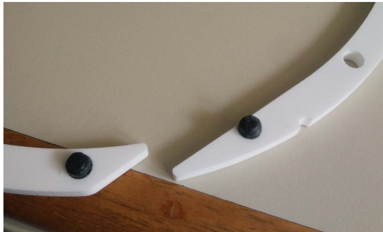
Figure 4.5.: Detail shot of one of the plastic rings used to secure the fibre bundles in place. The black parts are the plastic bolts used to mount the rings to each other.
