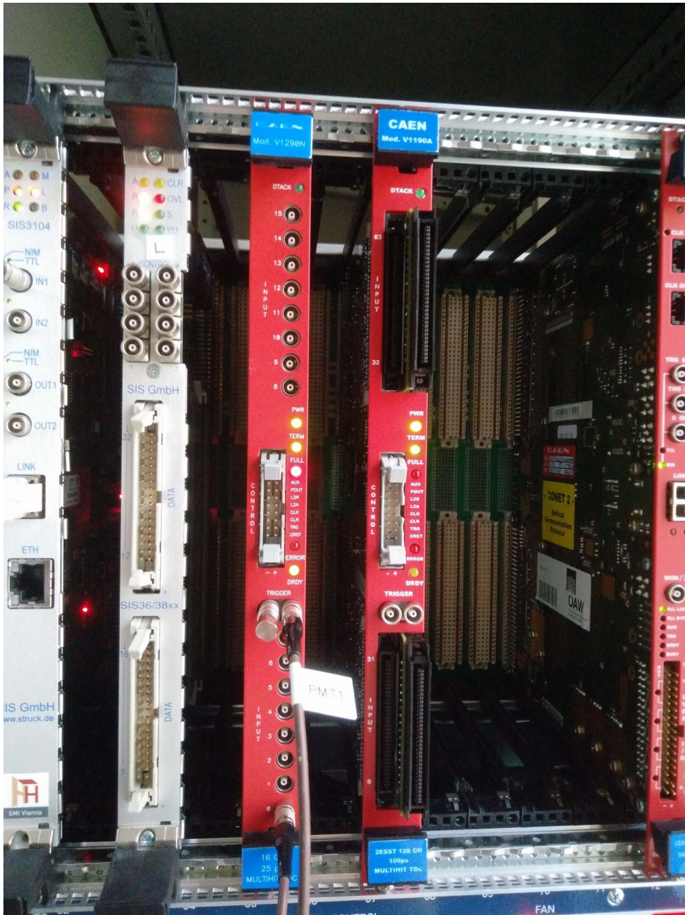
Figure 5.2.: The DAQ setup used for early testing, from the left: SIS3100 controller, SIS3820 scalar, V1290N TDC, V1190A TDC. On the rightmost side a V1742 module is shown, however, this was excluded from the test software due to unresolved hardware errors.
