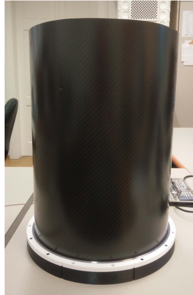
(b) The outer carbon tube. The upper end is bare, on the lower end the end piece and a ring used to secure the fibre bundles are mounted.
