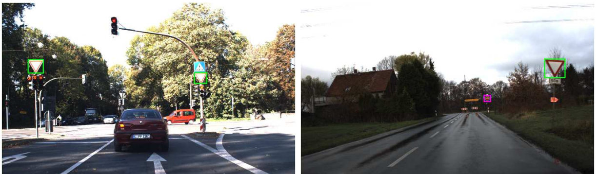
Figure 3.1: Example images of the GTSDb dataset. The annotated traffic signs are highlighted in green and purple. The bounding box of the stop sign (purple) has a size of 32 \times 32 pixels. Note: The GTSDb contains only annotations for prohibitory (including speed limits), mandatory and warning signs as well as stop and give way signs. Thus, the blue pedestrian crossing sign in the left image is not annotated.
