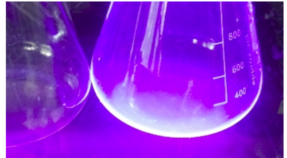
Figure 28. Sketch of a Erlenmeyer flask used in Shake Flask Fermentations, designating potential HFB fixation sites. Green represents the medium, blue represents mycelia, and the dotted line represents foaming (left). A shake flask fermentation containing mutants with a florescent hydrophobin tag showing significant binding of hydrophobin proteins to the glass post-removal of the medium. An empty Erlenmeyer flask adjacent provides a negative control (right).
