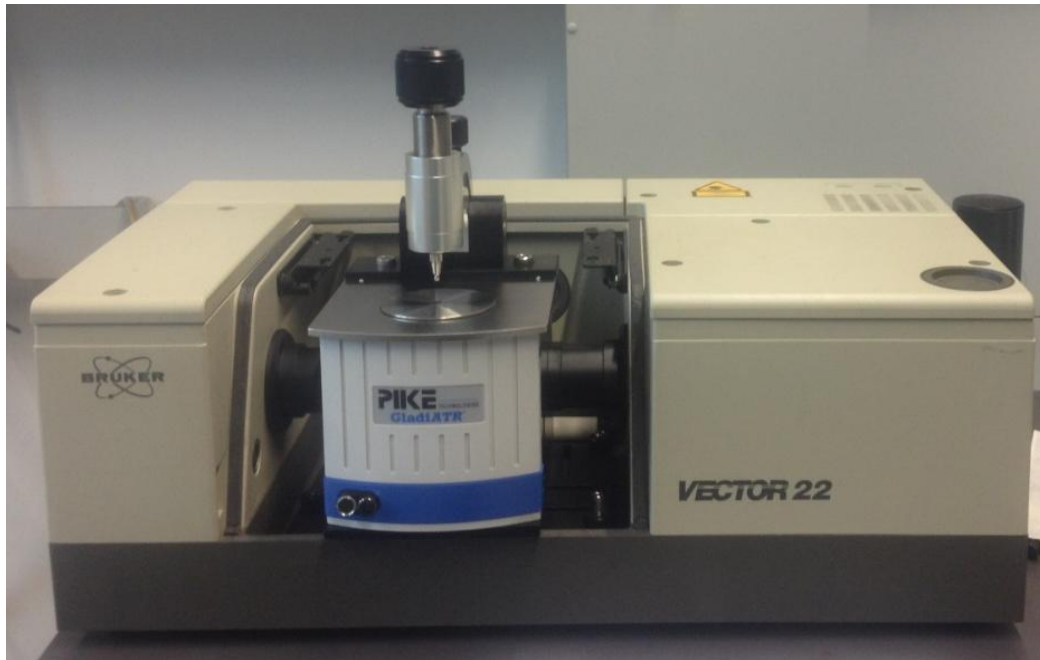
Figure 23: Bruker Vector 22 FTIR spectrometer with a PIKE GladiATR cell.
