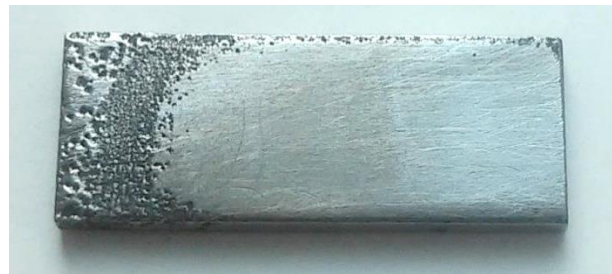
Figure 5.41 P9 steel after 240 h at 680 °C in the 100:0 gas atmosphere, cleaned
