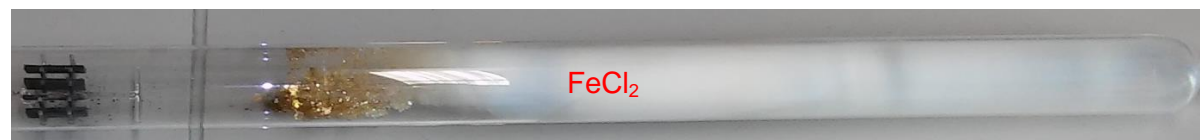
Figure 5.20 Re-crystallized \text{FeCl}_2 in the silica glass pipe after 240 h at 580 °C
