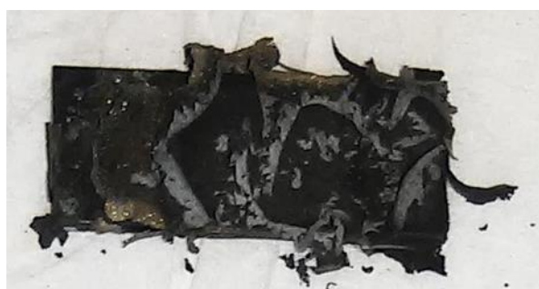
Figure 5.11 Alloy 800HT after 240 h at 480 °C in the gas atmosphere with HCl, after exposure to ambient atmosphere
