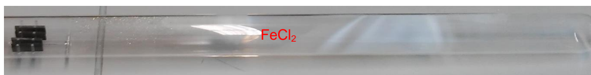
Figure 5.13 Re-crystallized \text{FeCl}_2 in the silica glass tube after 72 h at 480 °C
