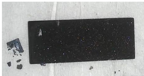
Figure 5.12 P9 steel after 240 h at 480 °C in the gas atmosphere with HCl
