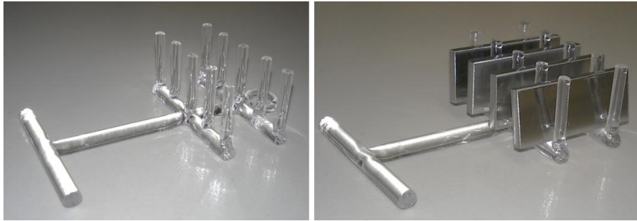
Figure 4.4 Silica glass holder without and with samples
