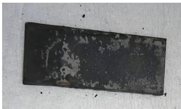
Figure 5.18 Alloy 800HT after 240 h at 580 °C in the 50:50 gas atmosphere
