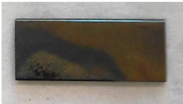
Figure 5.33 Alloy 800HT after 240 h at 480 °C in the 100:0 gas atmosphere
