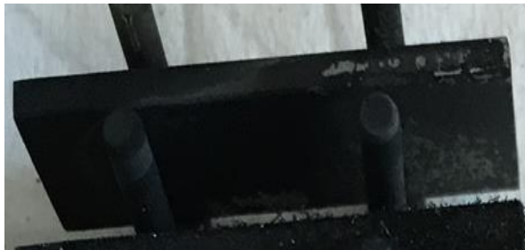
Figure 5.25 Alloy 800HT after 72 h at 680 °C in the 50:50 gas atmosphere
