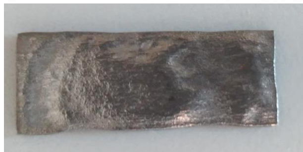
Figure 5.27 P9 steel at 680 °C after 72 h in the 50:50 gas atmosphere, cleaned
