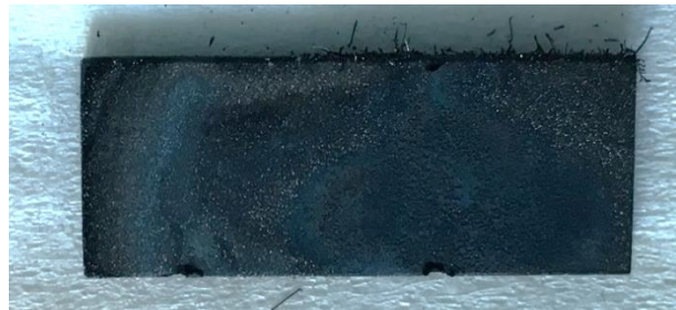
Figure 5.26 P9 steel after 72 h at 680 °C in the 50:50 gas atmosphere
