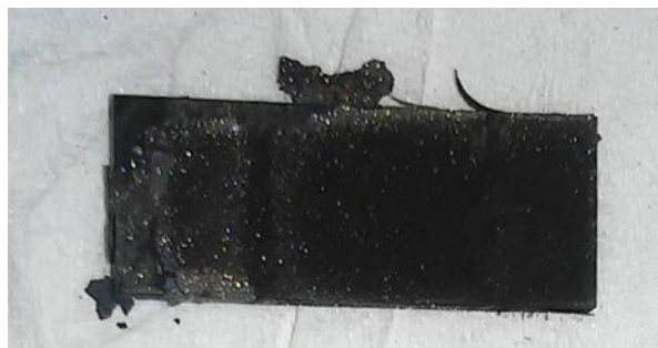
Figure 5.10 Alloy 800HT after 240 h at 480 °C in the gas atmosphere with HCl
