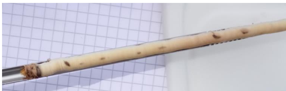
Figure 21: Picture of a drill core. The left end marks die outside of the tree.
