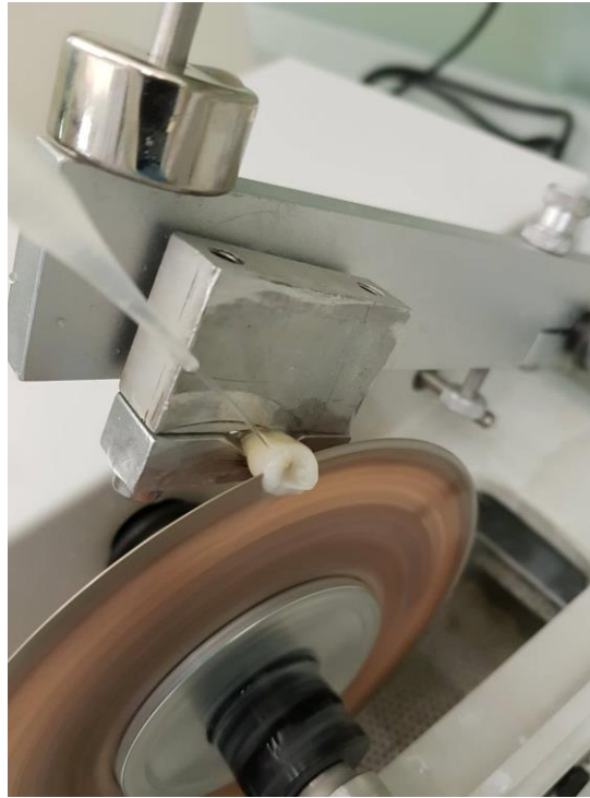
Figure 15 – Cutting of human tooth fixed to sample holder. This process was realized under continuous manual distilled water cooling.
