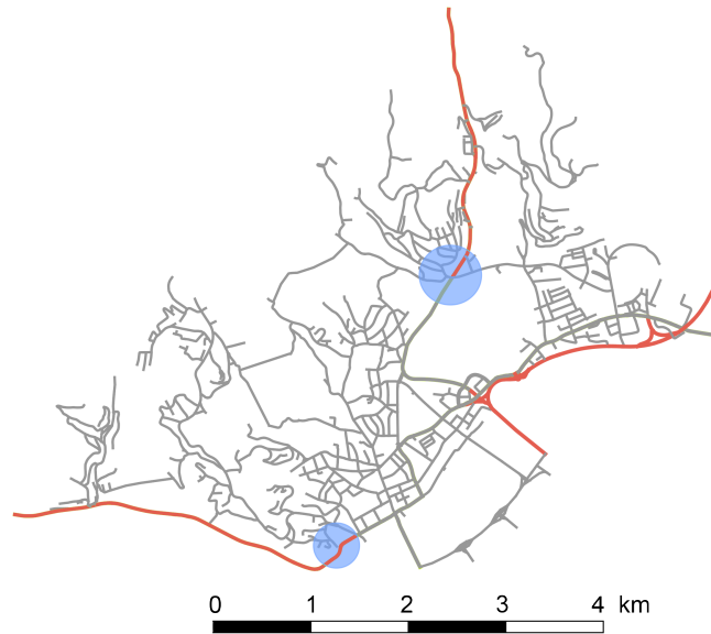
Figure 6.6: Simulated road network representing an extract of the city of Linz in Austria. Blue circles indicate potential bottlenecks in the road network which may cause a significant breakdown of traffic flow given a sufficiently high traffic density. High level roads such as freeways or expressways (speed limit 80-130 km/h) and low-level roads (30-50 km/h) are colored in red and gray, respectively.
