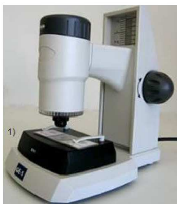
Figure 3.4: Digital Viewer GE-5 where 1) is the removable sample holder [41]
