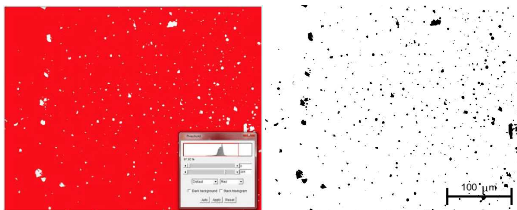
(c) Adjust Threshold until red covers residual layer completely.
