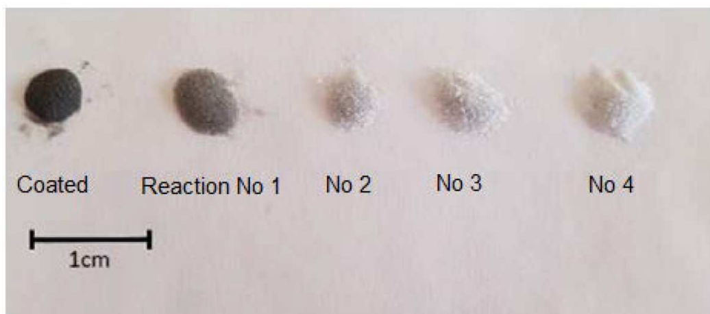
Figure 4.7: The originally dark-grey, sputter-coated HGMS get lighter after every hydrolytic reaction until they are almost white, which is the color of uncoated HGMS.
