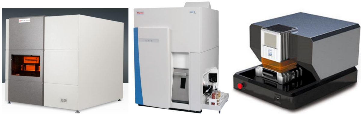
Figure 3.1: Tandem J200 LIBS instrument (left), iCAP SQ-ICP-MS instrument (center) and NWR 213 LA unit (right).
