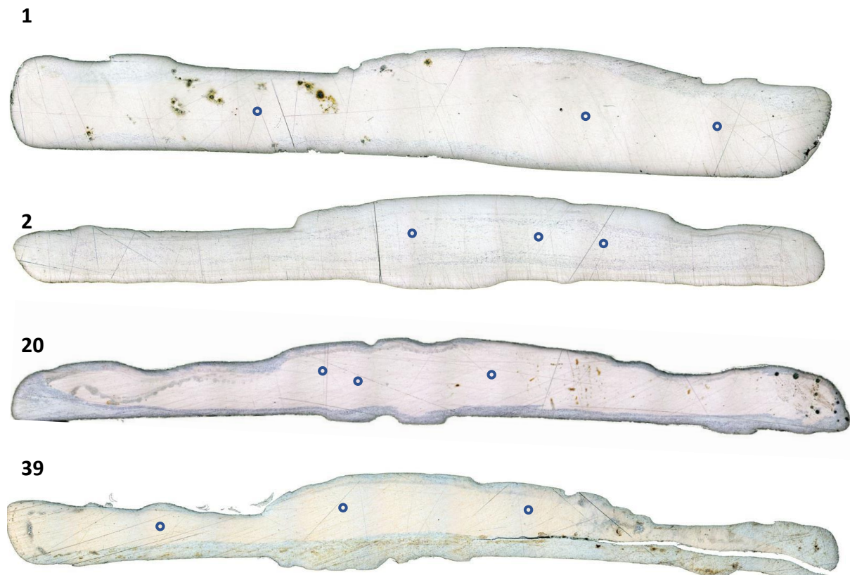
Figure 4.9: Microscopic images of the coins (no. 1, 2, 20, 39) used for comparison of the core alloy (Figure 4.10). The measured spots are marked by blue circles.
