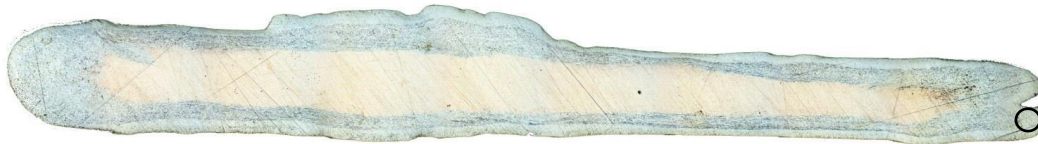
Figure 4.3: Microscopic image of coin no. 53 (COS V, approx. AD 110) with measurement spot marked as black circle. The corresponding spectra is shown in Figure 4.5 and enlarged sections of interest in Figure 4.5.
