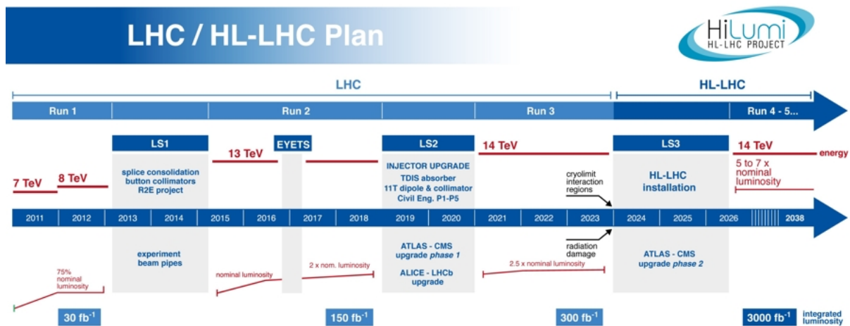
Figure 1.1.: Roadmap of the LHC showing the steps towards HL-LHC. LS1, LS2 and LS3 are so-called long shutdowns which are, together with the year-end-technical-stops (YETS), the only possibility to upgrade the machine. An extended YETS (EYETS) was needed after 2016 in order to upgrade cooling, vacuum and other cryogenic facilities. The two biggest detectors, ATLAS and CMS, are upgraded in two phases during LS2 and LS3. Picture taken from [1]
