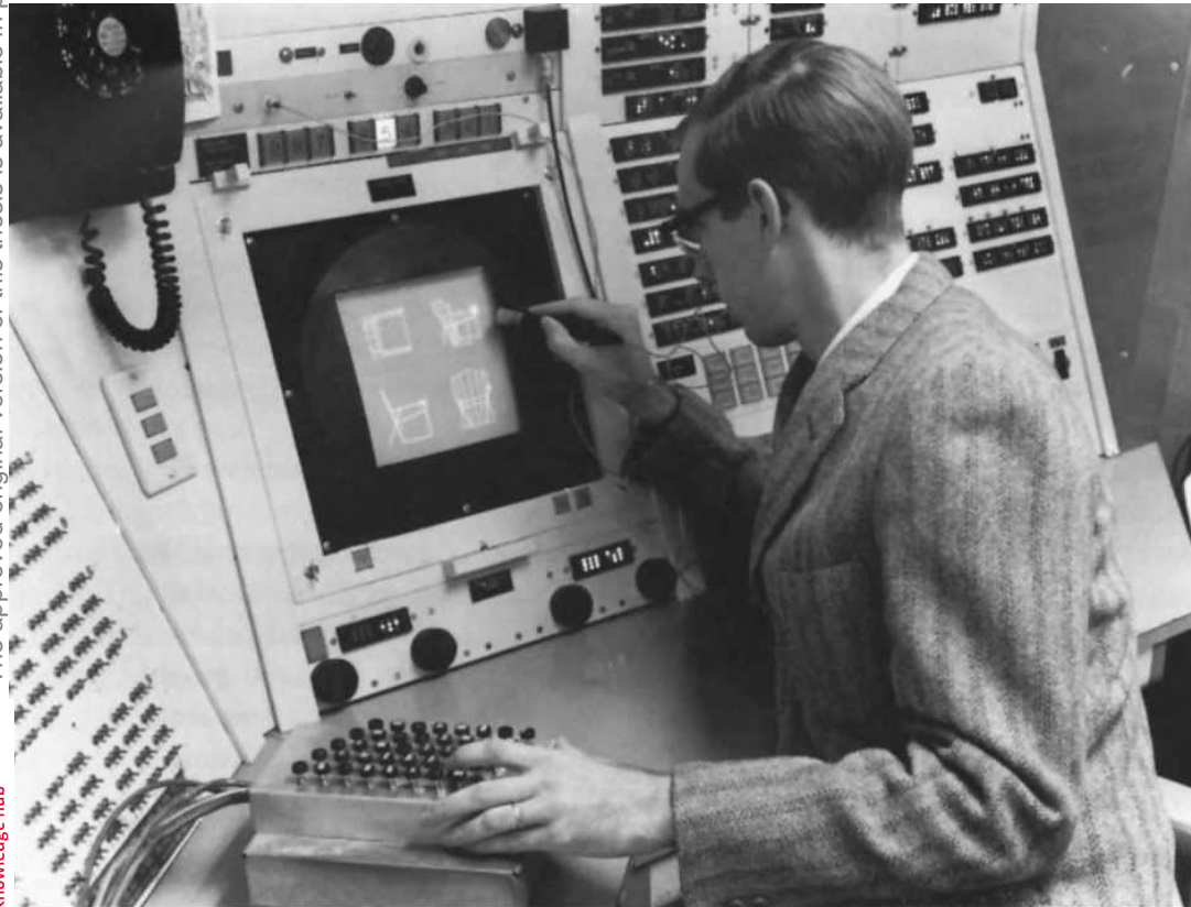
Figure 03. Ivan Sutherland's Sketchpad: Using a „light pen“, a Sketchpad user sketches directly on the screen and can both position parts of the drawing on the display or point to them to change them.
