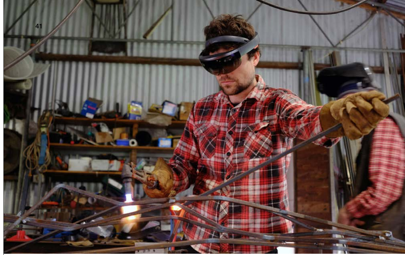
Figure 11. Augmented Robotics: Mixed reality environments for on-demand fabrication, assembly and analysis of complex steel structures. Figure 12. Brass Swarm, Shanghai, installation, 2015
