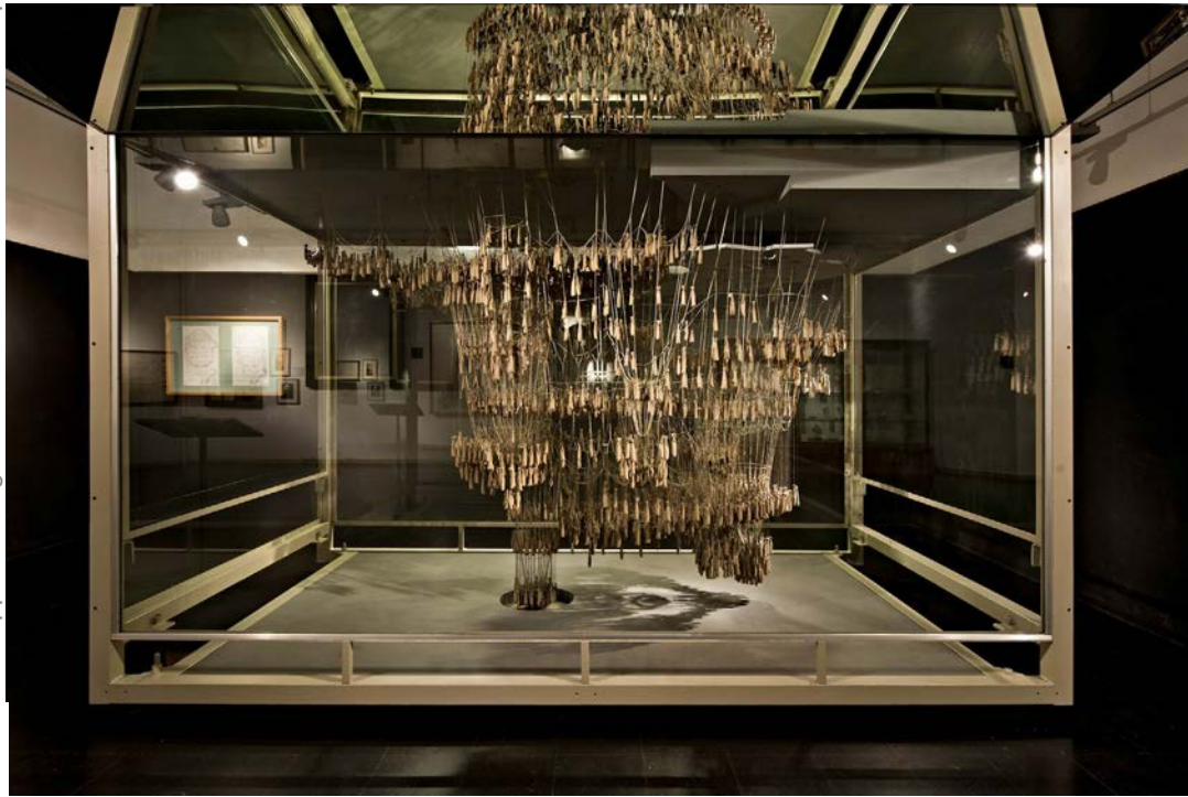
Figure 05. Hanging chain model by Antonio Gaudi, for Sagrada Familia in Barcelona.
