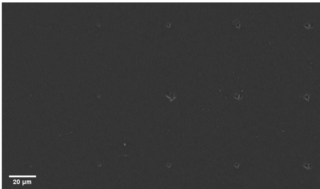
Figure 20: Arrangement of the measurement impressions on AlMgB 14 ( T_s = 600 °C) with a force from 50 mN (left) to 450 mN (right)
