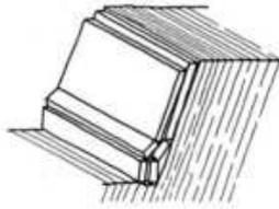
**Buckling of column- or slab-shaped rock blocks**
