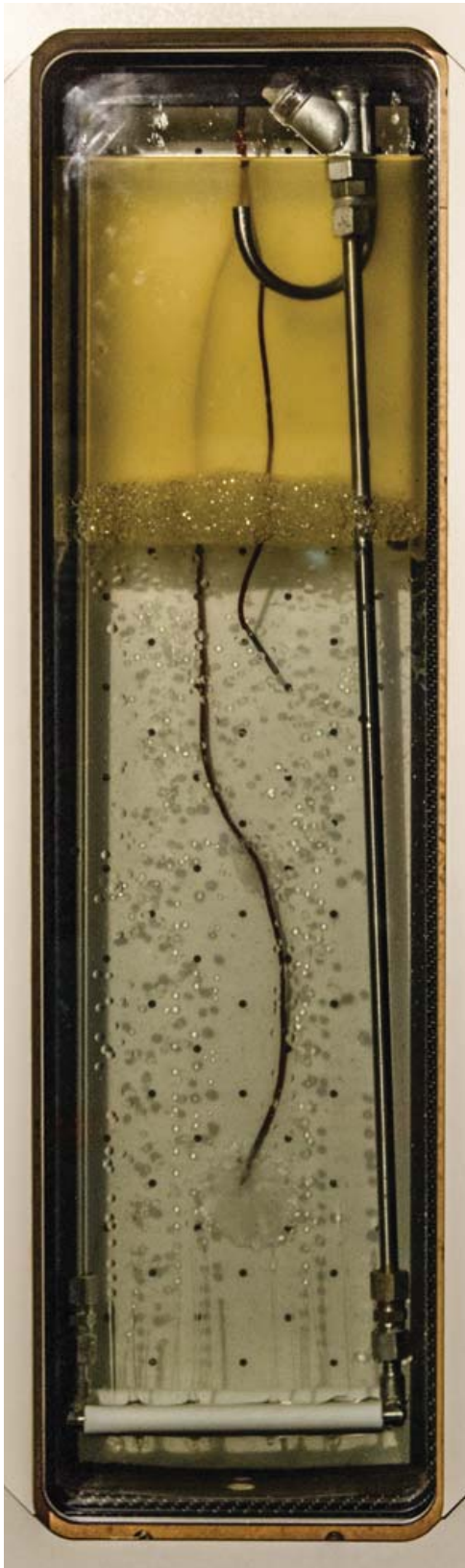
Figure 6: Strong foaming, crystallization around temperature sensors, cables[9]
