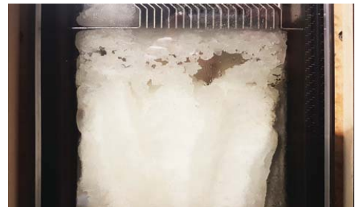
Figure 8: Solidification of PCM, pushed to top from HTF[9]
