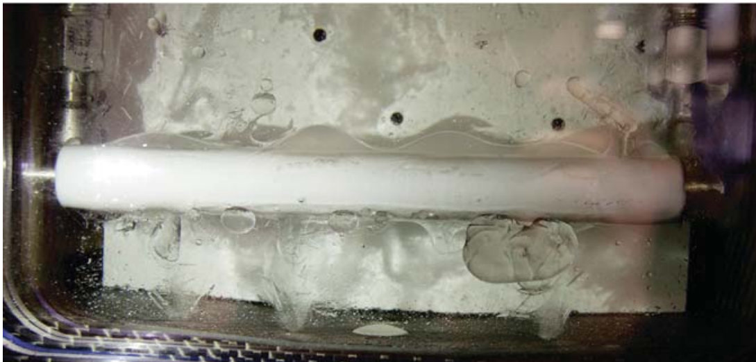
Figure 4: Image showing the frozen heat exchanger due to water drifting alongside ADX10 [9]
