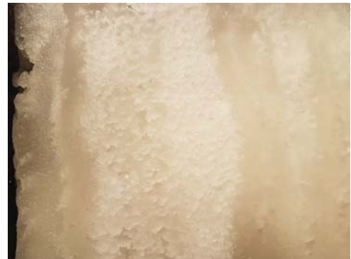
Figure 7: Conduits left behind by HTF, porous structure[9]
