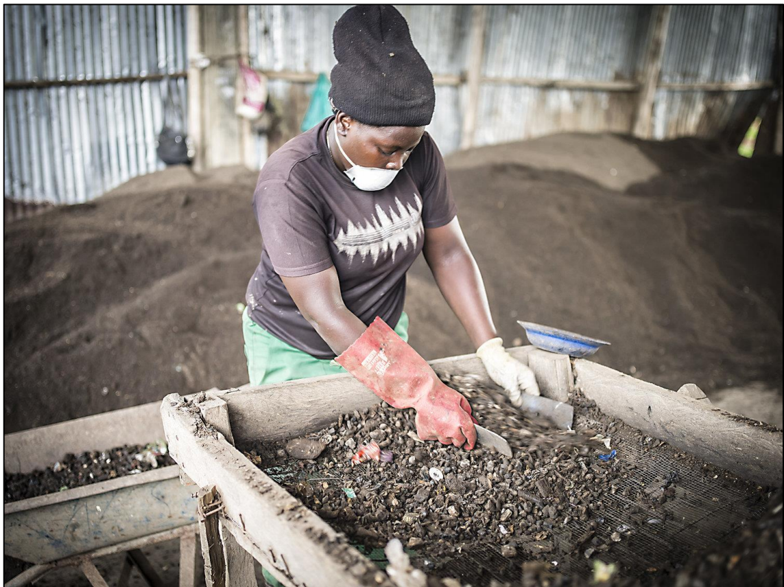
Figure 1.9: Compost purification via sieving at the Mukono composting plant SOURCE: The Uganda Waste Report, ©Timothy Bouldry, 2018
