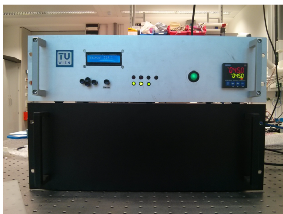
Fig. 4 Left: front side of the developed sensor (19" rack compatible); right: schematic assembly of the optical and electrical parts
