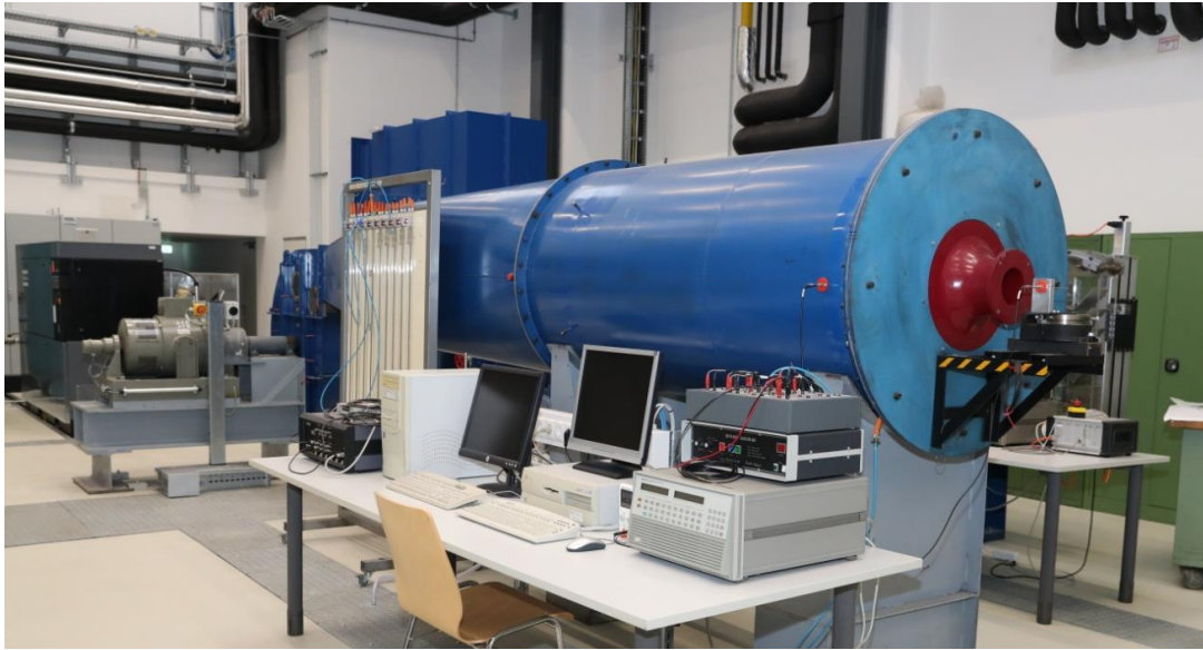
Figure B.3 Free jet facility with support devices at Institute for Energy Systems and Thermodynamics, Technische Universität Wien
