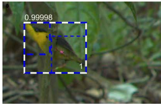
Figure 4.3: The two small blobs (small blue bounding boxes) are combined into a bigger blob (big blue bounding box). The white text indicates the blobs' target scores.
