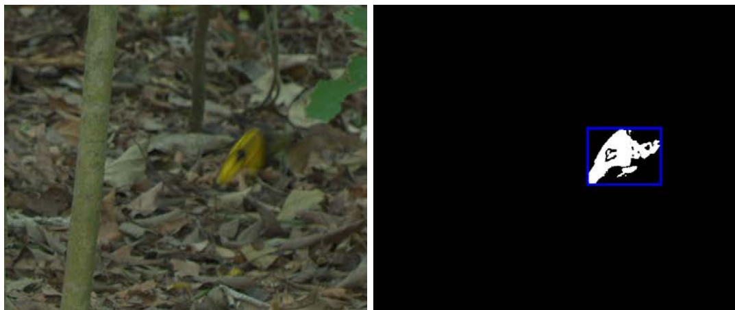
Figure 4.2: Foreground mask (right) generated by Mixture Of Gaussians model of frame (left). The blue box marks the extracted blob.
