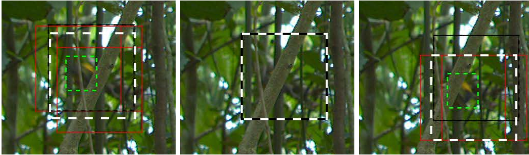
Figure 4.5: Middle: The Kalman filter’s location estimation (black box) is used as the bounding box output when the bird becomes invisible to the camera during a jump. Left, right: The bird is visible and can thus be recognized by the CNN. (green boxes: ground truth; red boxes: candidate locations classified as target; white boxes: bounding box output for current frame)
