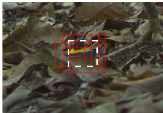
Figure 4.4: Bird is sitting and no blob was found (red box: candidate locations with target score \geq t_3 , white box: final bounding box)
