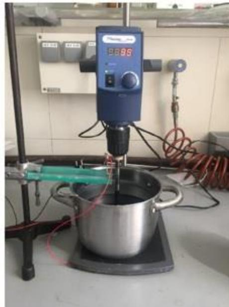
Fig. 3. 5: Equipment for electropolishing.
