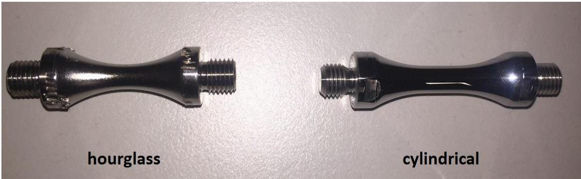
*Fig. 3. 6: End shape of specimens.*
