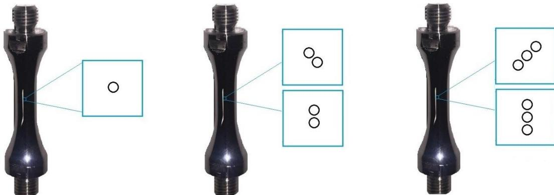
Fig. 3. 9: The orientation of difference holes.
