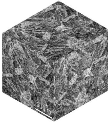
Fig. 3. 1: Martensitic microstructure of 17-4PH [15].
