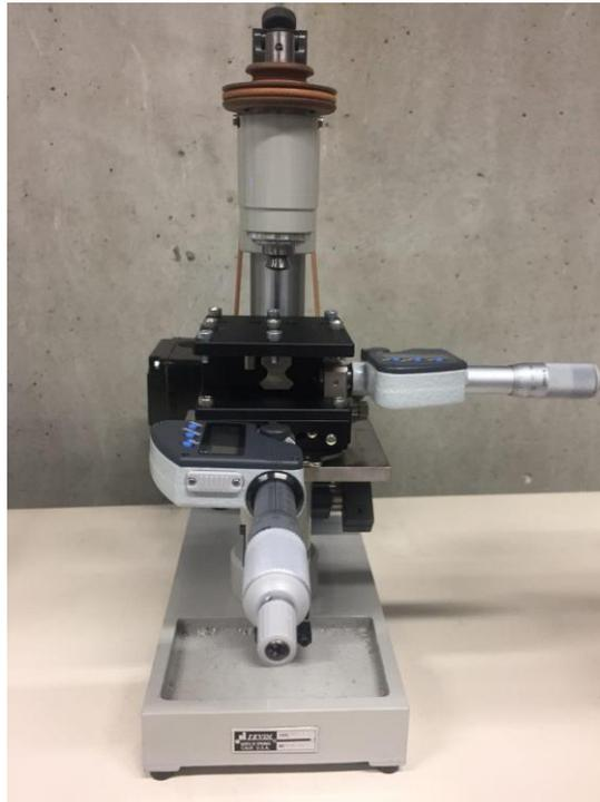
*Fig. 3. 7: Micro drill machine.*
