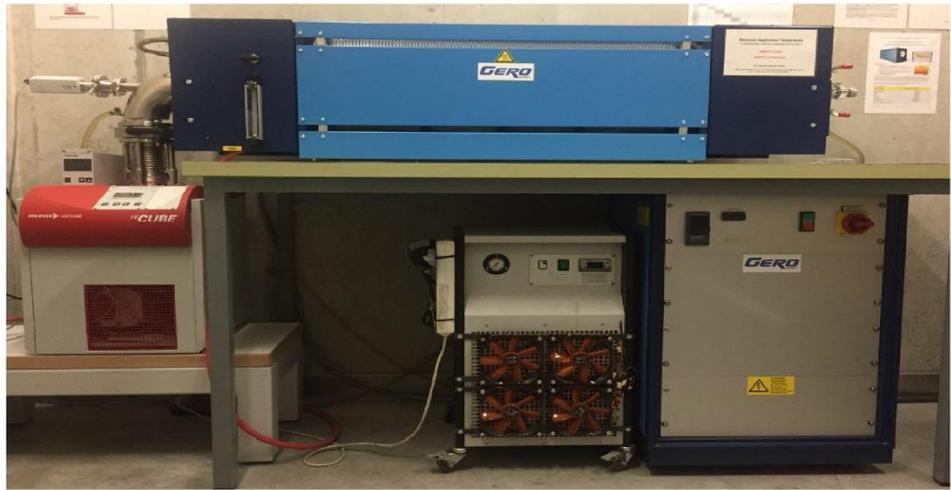
Fig. 3. 8: Oven and centrifuge pump used for residual stress relieving.
