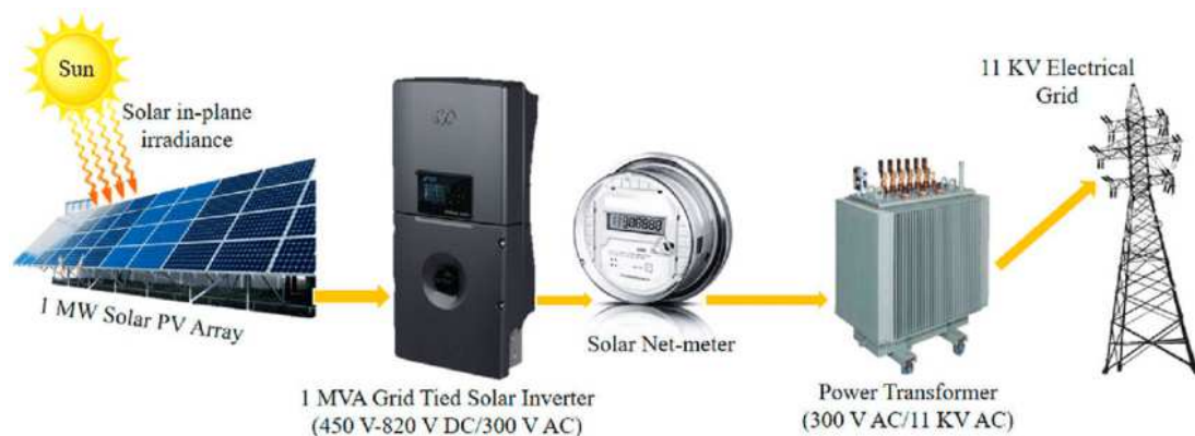
Figure 11 .- Transformer together with main components of a PV plant (Kumar (2017))
