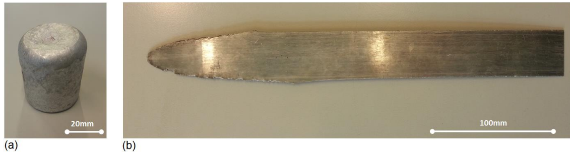
Figure 21: Opticast sample (a) and the used laboratory-made pure alloy after rolling (b).
