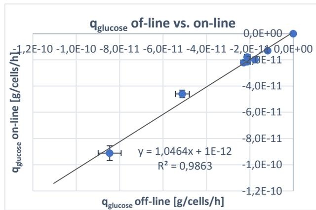
**Figure 16 Comparison of on-line and off-line determined specific glucose uptake rates.**
