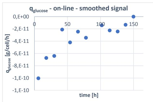
**Figure 15** Detection of glucose limitation using a smoothed on-line signal.
