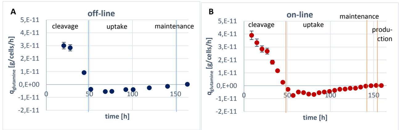
**Figure 13** Three different process phase can be distinguished concerning the glutamine metabolism: (A) off-line determined specific glutamine uptake rates; (B) on-line determined specific glutamine uptake rates.
