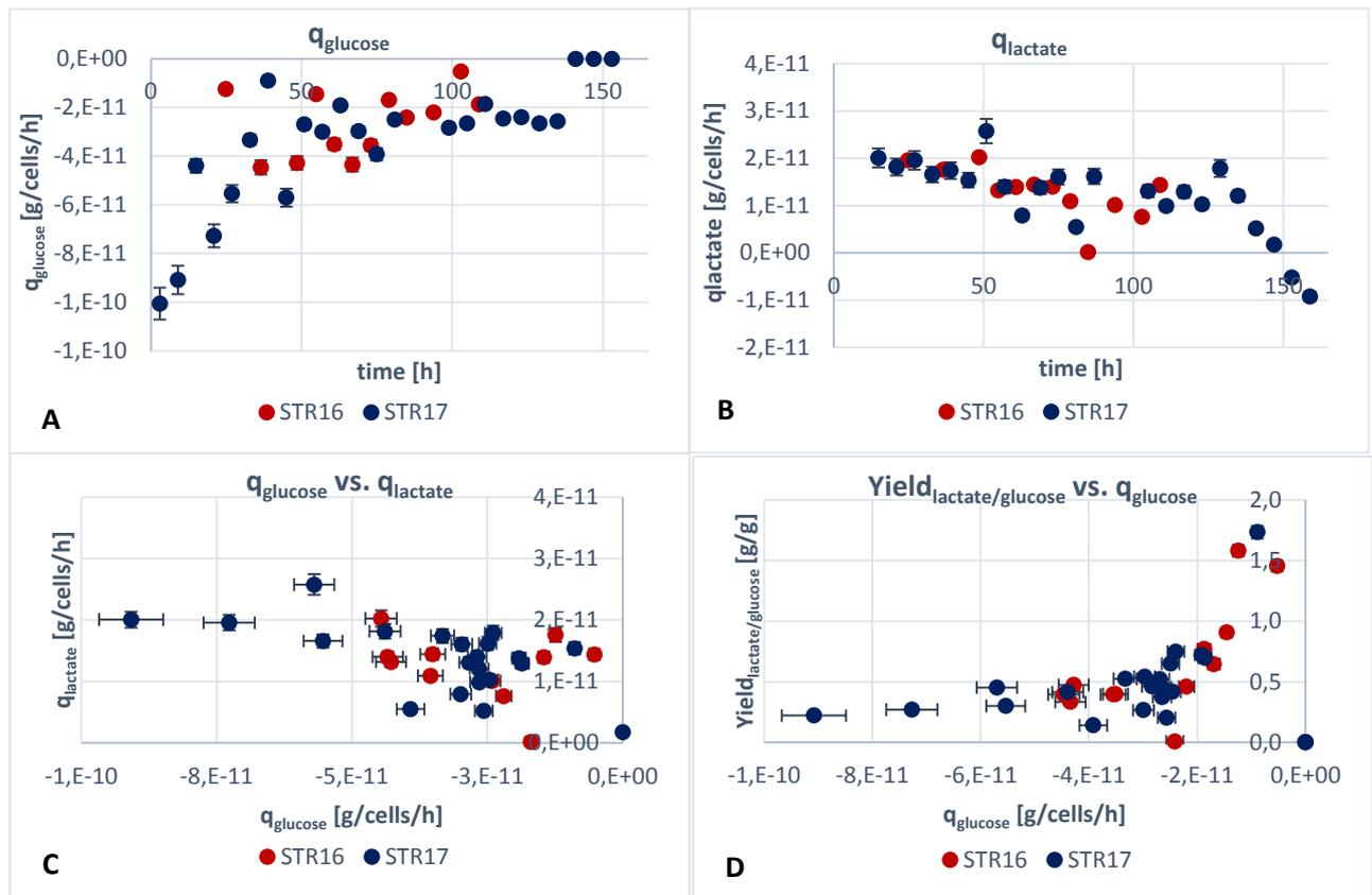
**Figure 19** Specific rates and yields for glucose and lactate comparing STR16 and STR17: (A) specific glucose uptake rate over time; (B) specific lactate production rate over time; (C) specific lactate production rate over specific glucose uptake rate; (D) Yield lactate/glucose plotted over the specific glucose production rate;
