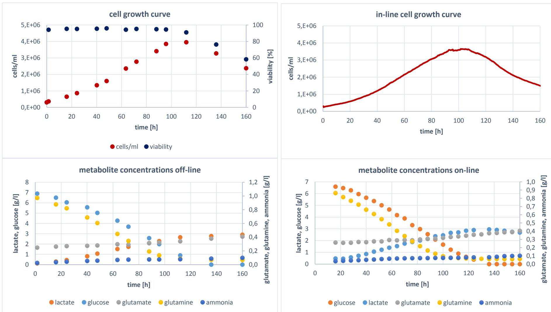
Figure 31 Acquired data of STR14: (A) viable cell count (red) and viability (dark blue); (B) in-line measured viable cell count; (C) off-line measured metabolite concentrations, orange, lactate; light blue, glucose; grey, glutamate; yellow, glutamine; dark blue, ammonia;
