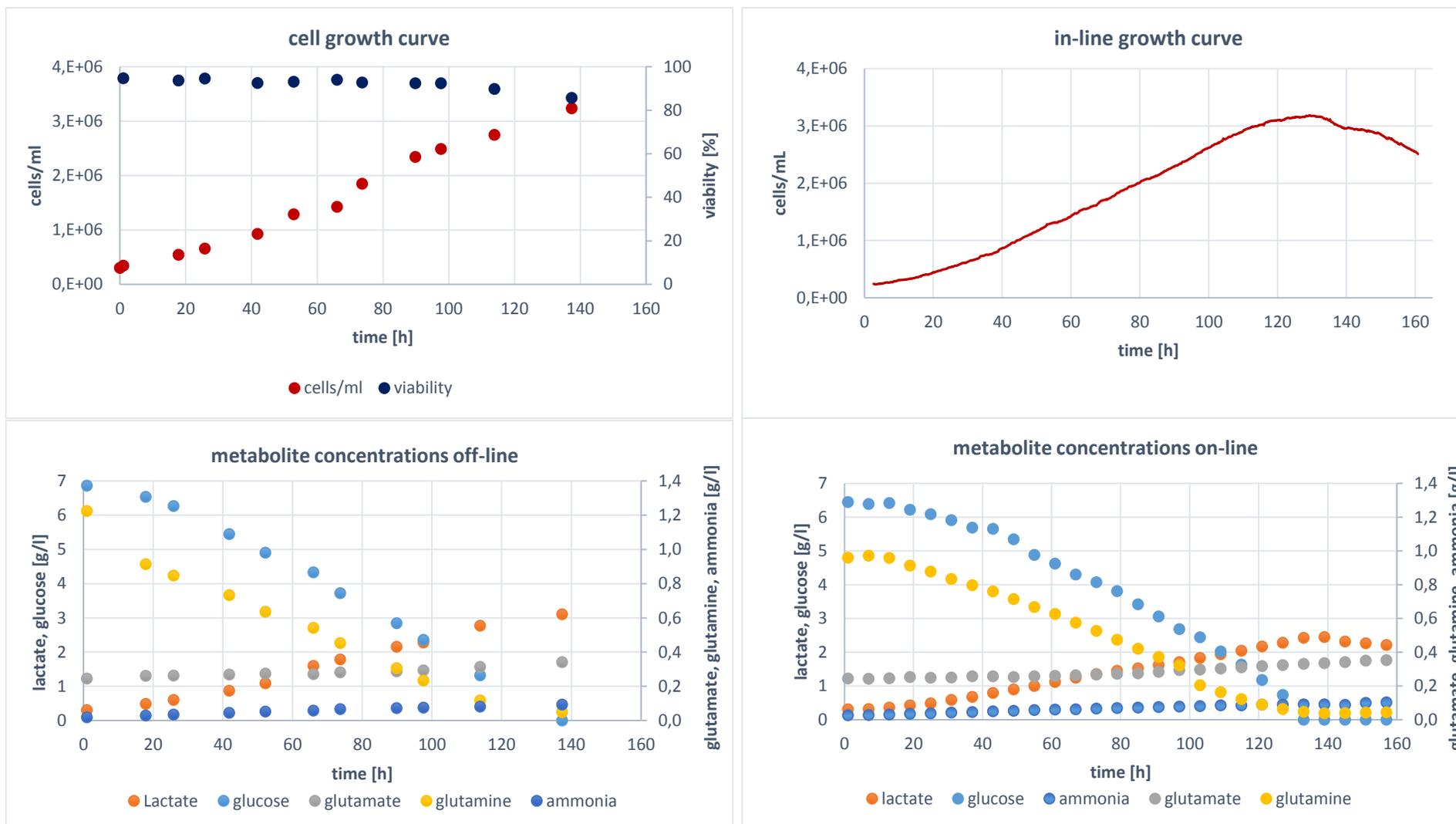
Figure 28 Acquired data of STR13: (A) viable cell count (red) and viability (dark blue); (B) in-line measured viable cell count; (C) off-line measured metabolite concentrations, orange, lactate; light blue, glucose; grey, glutamate; yellow, glutamine; dark blue, ammonia;
