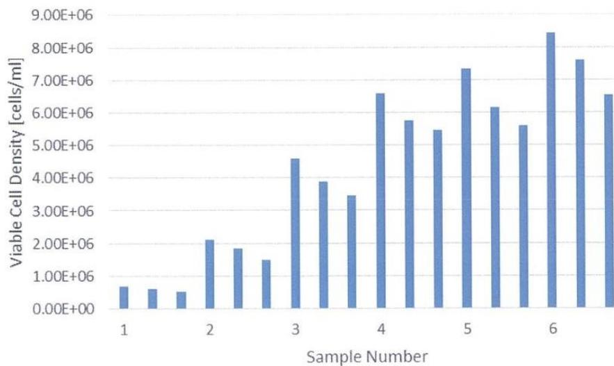
**Figure 2:** Cedex cell count in triplicates per time point. Cell number decreases per measurement point as cells adhere to the surface of the Cedex sample cups.
