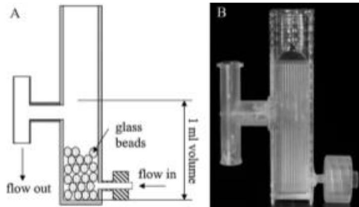
**Figure 4 Construction of the flow- through cuvette: (A) schematic illustration; (B) picture of the cuvette (Dietzsch 2013).**
