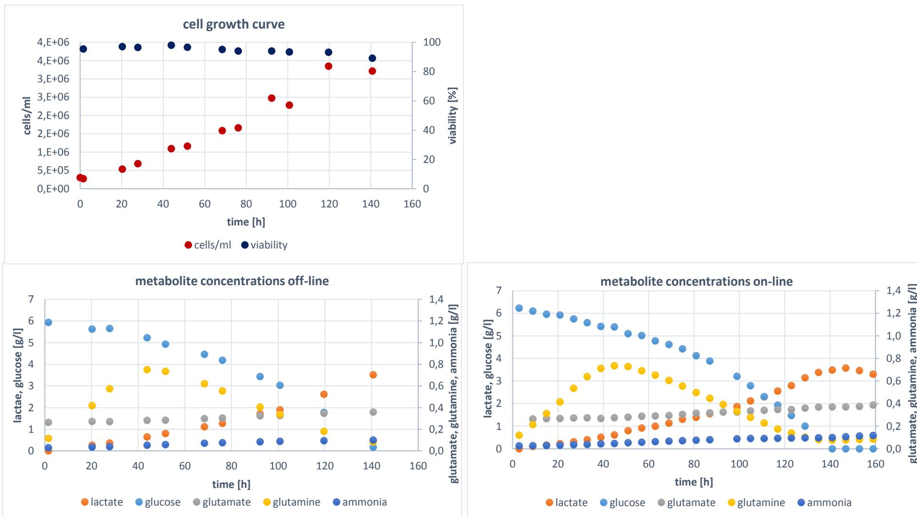
Figure 37 Acquired data of STR17: (A) viable cell count (red) and viability (dark blue); (C) off-line measured metabolite concentrations, orange, lactate; light blue, glucose; grey, glutamate; yellow, glutamine; dark blue, ammonia;
