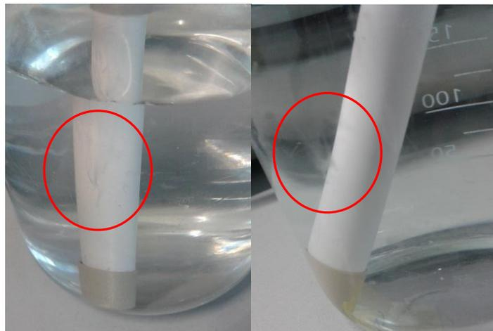
*Figure 5 Leakage of the membrane.*
