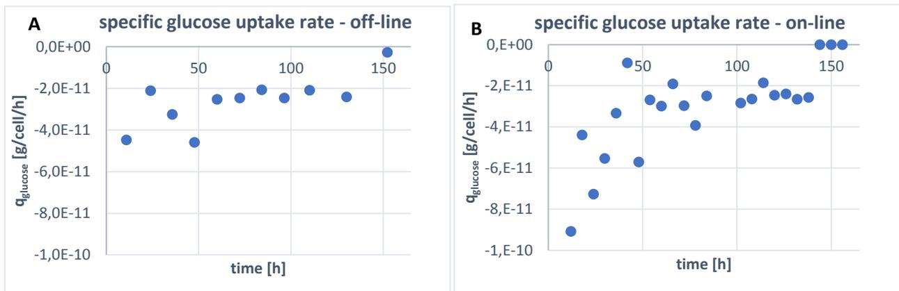
**Figure 14** Detection of glucose limitation using on-line and off-line glucose uptake rates: (A) off-line determined specific glucose uptake rate; (B) on-line determined specific substrate uptake rates.
