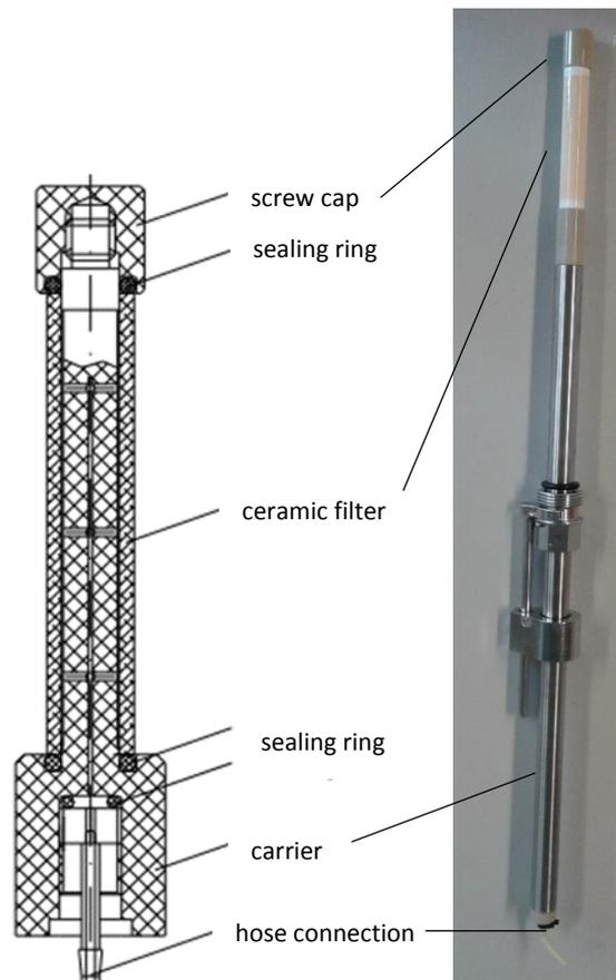
**Figure 6 Schematic scheme and picture of a filter membrane.**
