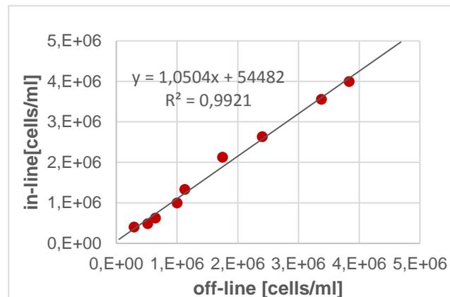
**Figure 9** Correlation between off-line viable cell counts and In-line permittivity data converted by the MLR model.
