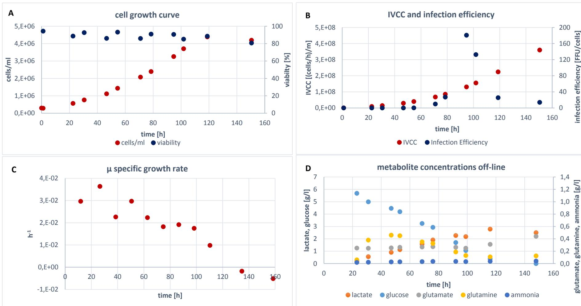
Figure 26 Acquired data of STR8: (A) Viable cell count (red) and viability (dark blue); (B) Integrated viable cell count (red) and Infection Efficiency (dark blue); (C) specific growth rate; (D) off-line measured metabolite concentrations, orange, lactate; light blue, glucose; grey, glutamate; yellow, glutamine; dark blue, ammonia;
