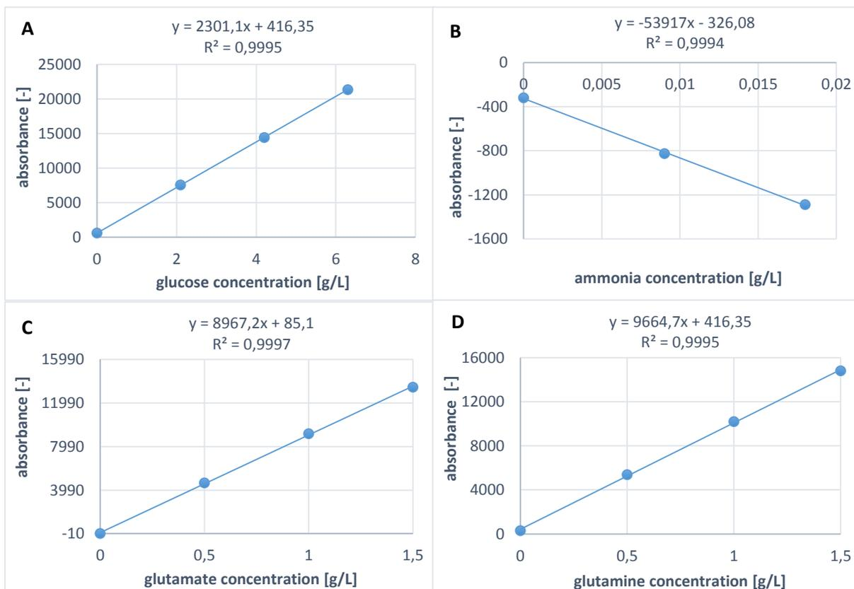
**Figure 25** Linear calibration range of the various substrates: (A) glucose; (B) ammonia; (C) glutamate; (D) glutamine;
