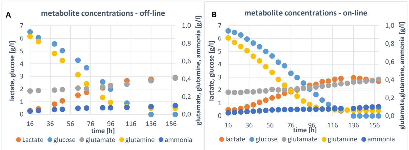
**Figure 12** Metabolite concentrations of STR14 measured using CuBiAn XC in off-line and on-line mode: (A) off-line; (B) on-line.
