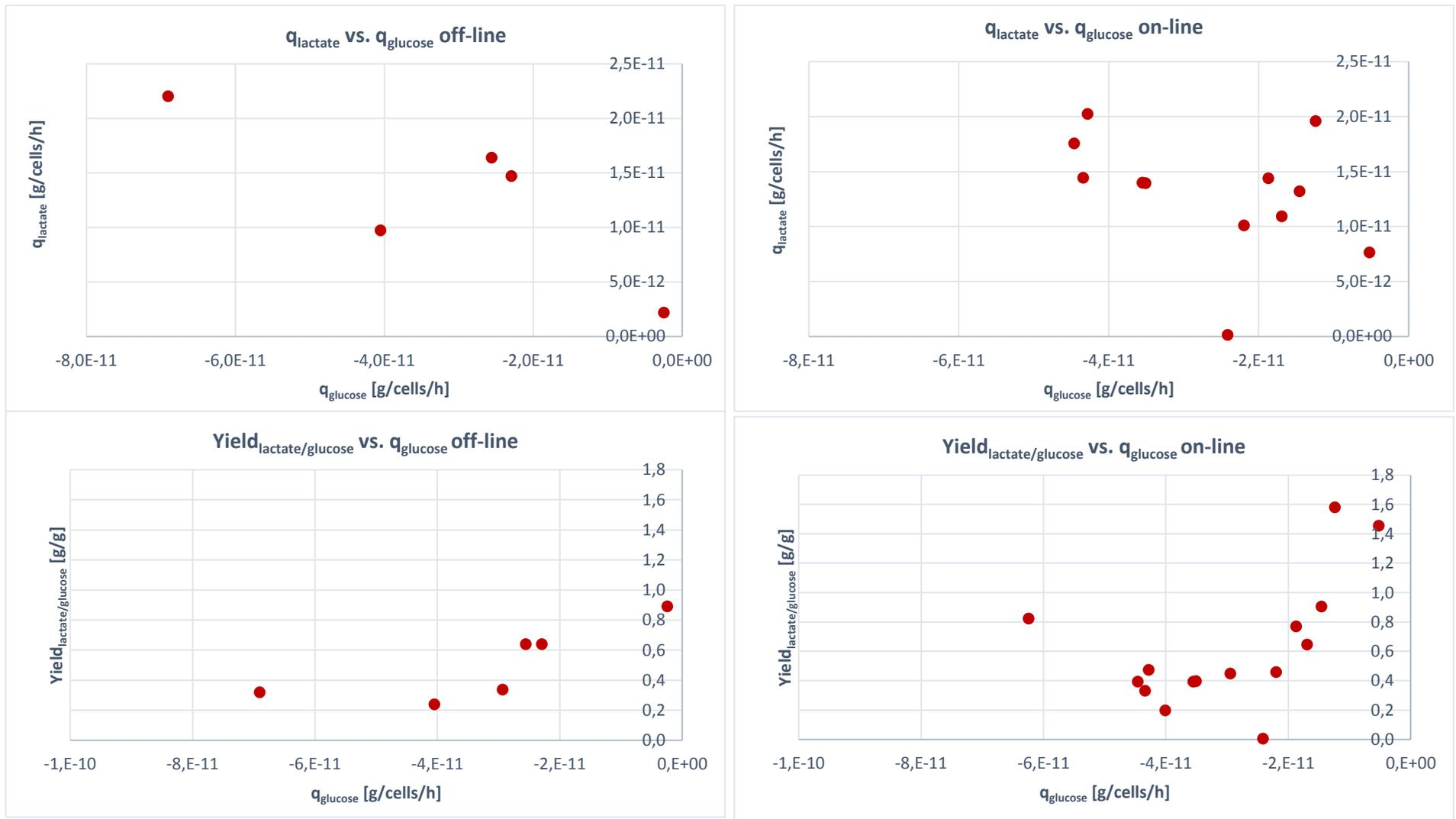
Figure 36 Specific rates and yields of STR16 plotted over the specific glucose uptake rate: (A) on-line determined specific lactate production rate; (B) off-line determined specific lactate production rate; (C) off-line determined Yield<sub>lactate/glucose</sub>; (D) off-line determined Yield<sub>lactate/glucose</sub>;
