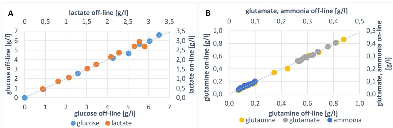
**Figure 11** Off-line measured metabolite concentrations of STR14 plotted over on-line measured one: (A) glucose and lactate; (B) glutamine, glutamate and ammonia.
