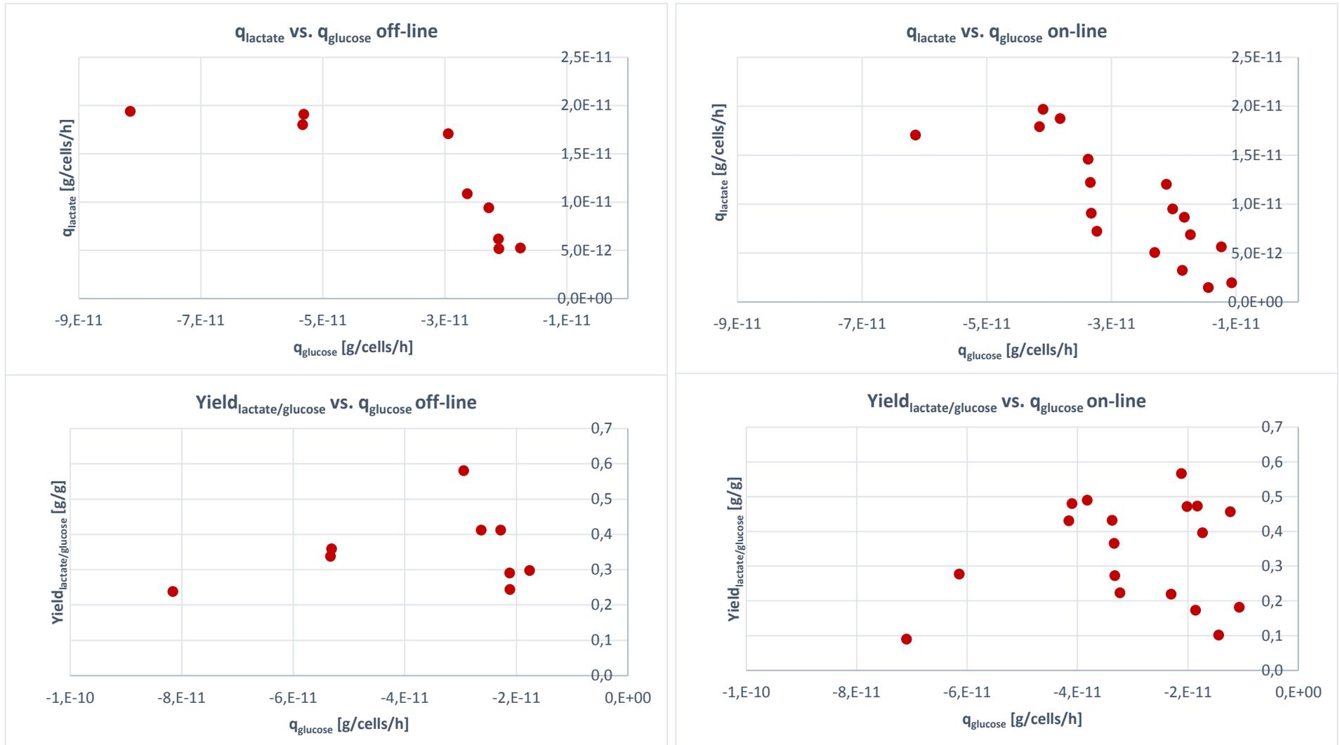
Figure 33 Specific rates and yields of STR14 plotted over the specific glucose uptake rate: (A) on-line determined specific lactate production rate; (B) off-line determined specific lactate production rate; (C) off-line determined  $Yield_{lactate/glucose}$ ; (D) off-line determined  $Yield_{lactate/glucose}$ ;
