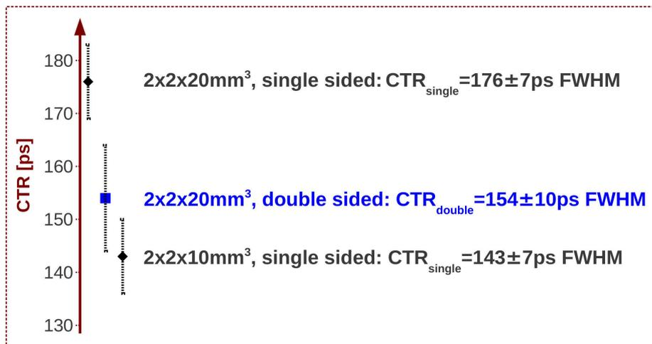
**Figure 9.8.:** Comparing single sided readout with double sided readout. The standard single sided readout measurements give 176ps FWHM CTR for 20mm long crystals. Whereas the time resolution improves to 154ps by using double sided readout of the same 20mm long crystal. In comparison 10mm long crystals readout single sided give a CTR of 143ps FWHM.
