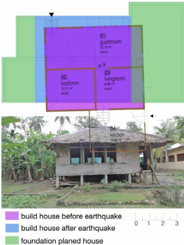
fig. 72: consequence of the earthquake 2005 at the house "ntumo 561"
