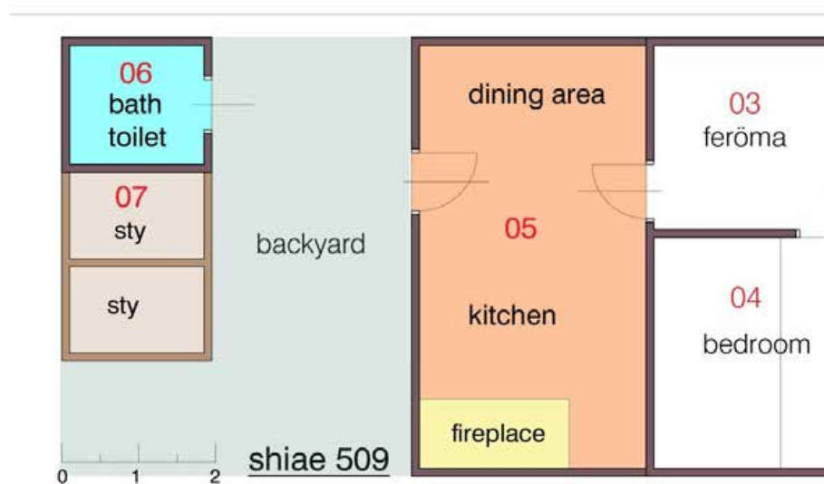
fig. 192: bathroom and toilet separated in the backyard "shiae 509"
