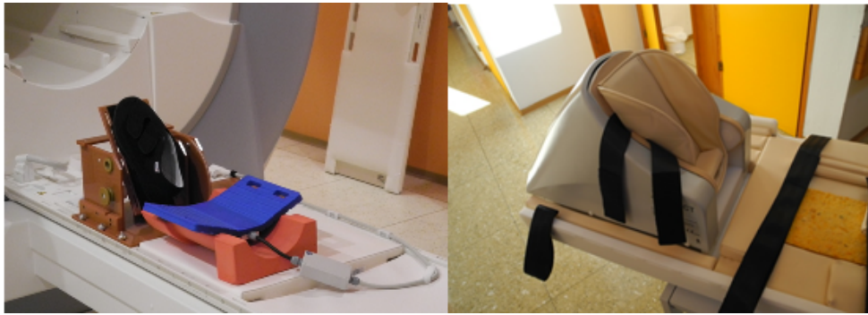
Figure 6.2: Left: Home-built ergometer with mechanical system used in first institute. Right: Ergospect ergometer with pneumatic system used in second institute.
