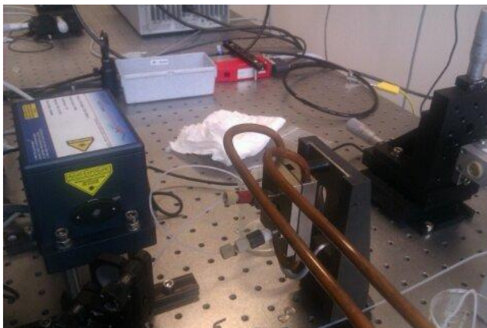
Figure 21 – Flow cell with temperature stabilized water circuit
