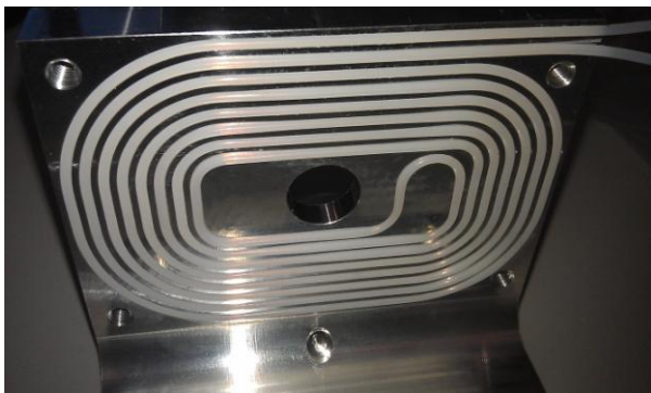
Figure 22 – Meander with the temperature-stabilized tubing
