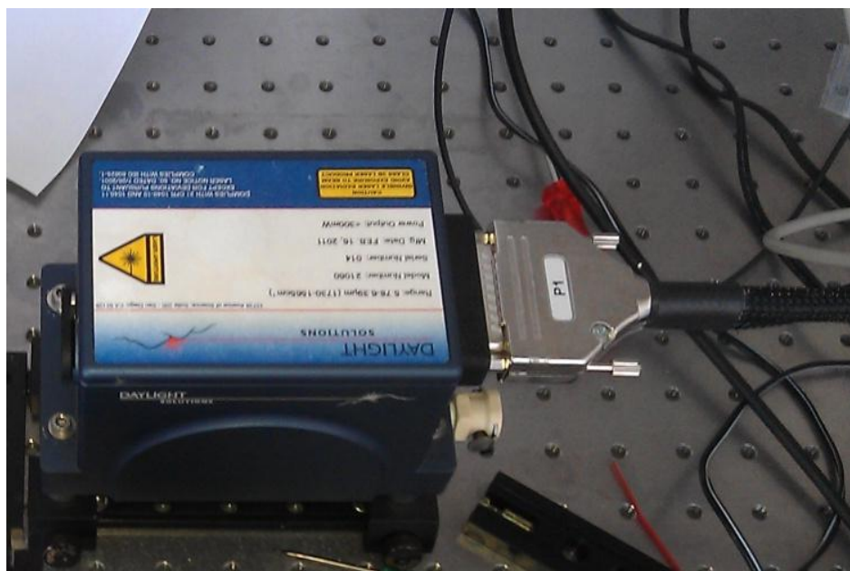
Figure 17 – EC-QCL from Daylight Solutions ( 1565.06\text{-}1729.30\text{cm}^{-1} )
