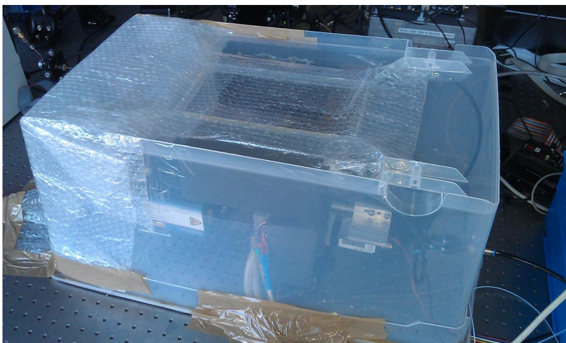
Figure 16 - Setup with a dry air purged hood
