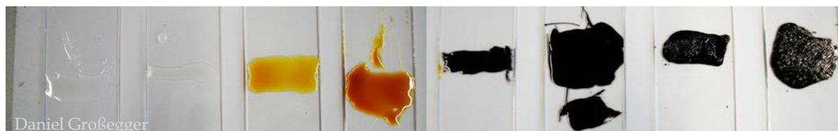
Figure 26: Two prepared samples of saturates, aromatics, resins and asphaltenes (right to left)
