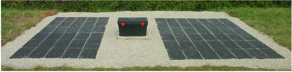
Figure 19: Test field: with snow service (right) and without snow service (left) of unmodified (back) and modified (front) test pieces [23]
