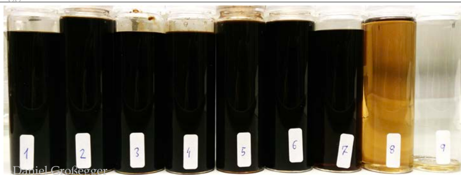
Figure 32: Weight per cent distribution and snap-cap vials of asphaltenes (obtained from B) separated by liquid column chromatography
