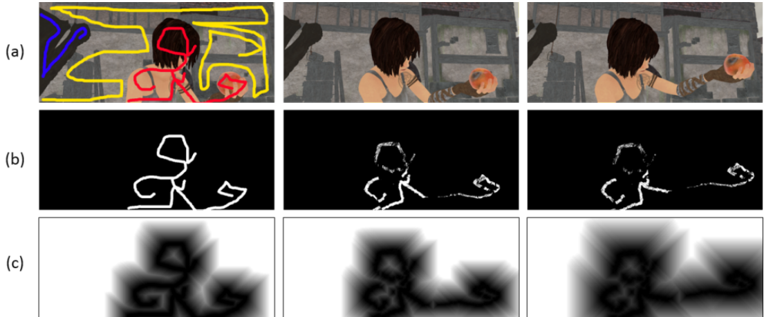
Figure 4.5: (a) shows frame 1, 13 and 20 (from left to right) of the input video. (b) presents the movement of points belonging to the red coloured scribble in the first frame by showing their long motion path pixels in frame 1, 13 and 20. (c) visualizes the distance maps with a spatial threshold t_{spatial} = 100 . Black pixels are the tracked scribble points of scribble l , while white pixels result in total costs of 0. Grey values in between are reducing linearly the colour probability c_{col}(i, l) and result in higher total costs.
