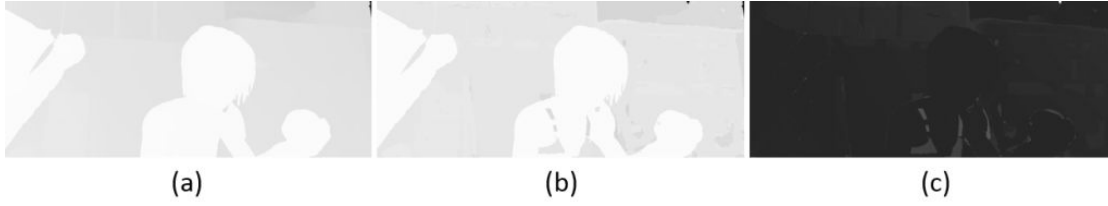
Figure 5.3: (a) Depth ground truth, (b) resulting depth map using our proposed algorithm, and (c) difference to depth ground truth. The lighter a pixel is, the higher is the difference at this pixel.
