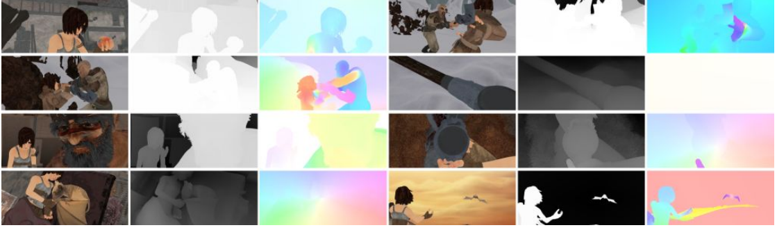
Figure 5.1: Test videos from the MPI-Sintel data set [16]. The first frame, the corresponding depth ground truth and corresponding optical flow ground truth of the eight test videos used in the evaluation are shown. Test videos (from left to right, two test videos in a row): alley1 , ambush2 , ambush5 , ambush7 , shaman2 , shaman3 , sleeping1 and temple3 .
