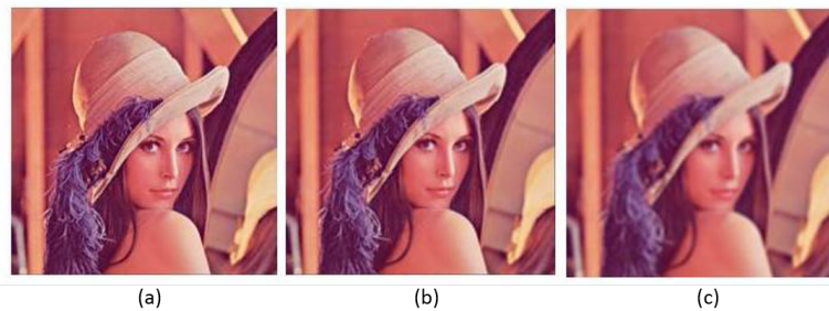
Figure 3.4: Linear filtering with a box filter: (a) input image, (b) filtered with a 3 \times 3 box filter and (c) filtered with an 8 \times 8 box filter. Because of the larger filter kernel in (c) the image is smoother, but diffuse.
