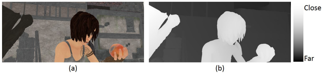
Figure 1.1: (a) Input image and (b) corresponding depth map. The depth values are presented as grey values from dark (far) to white (close). [16]
