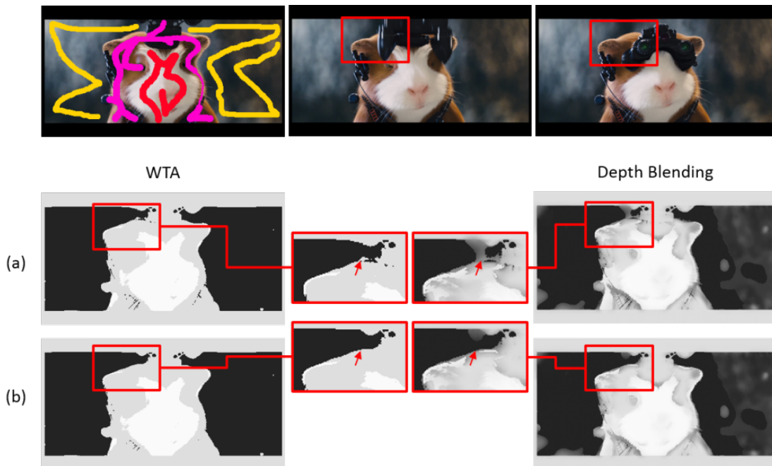
Figure 4.4: Comparison of the naive extension of [11] of Section 4.1 shown in (a) and the results of the temporal consistency improvement shown in (b). To the left the resulting depth propagation using the WTA approach is shown, while to the right the resulting depth propagation using the depth blending is shown. As can be seen, the noise especially at depth borders is being reduced.
