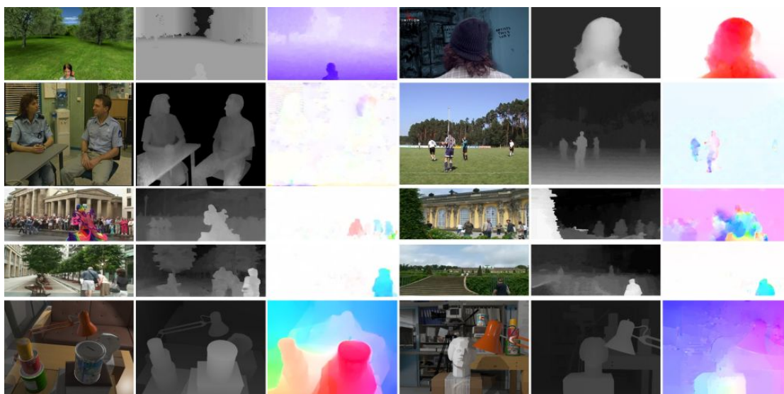
Figure 5.2: 10 of 11 test videos used to compare resulting depth maps with [42]. The first frame, the corresponding depth ground truth/reference depth and corresponding optical flow ground truth/estimated optical flow of the test videos used in the evaluation are shown. Test videos (from left to right, two test videos in a row): Child [10], Head [10], Interview [10], Soccer [12], Parade [12], Palace [12], City [12], Staircase [12], Tsukuba380-397 [56] and Tsukuba50-66 [56].
