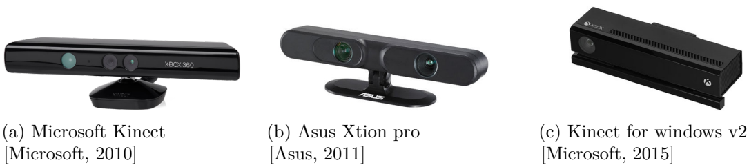
Figure 2.12: Versions of the Kinect sensor
