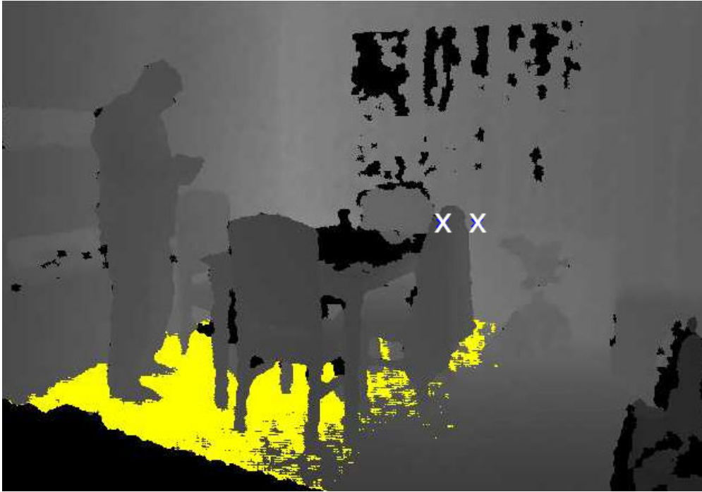
Figure 3.4: ROI (dataset 1): depth image with the ground floor marked yellow, ROI marked as X
