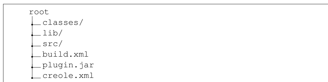
Figure 4.2: Directory structure of a processing resource
