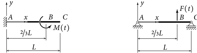
(a) Cantilever beam with harmonic moment. (b) Simple supported beam with harmonic force.
