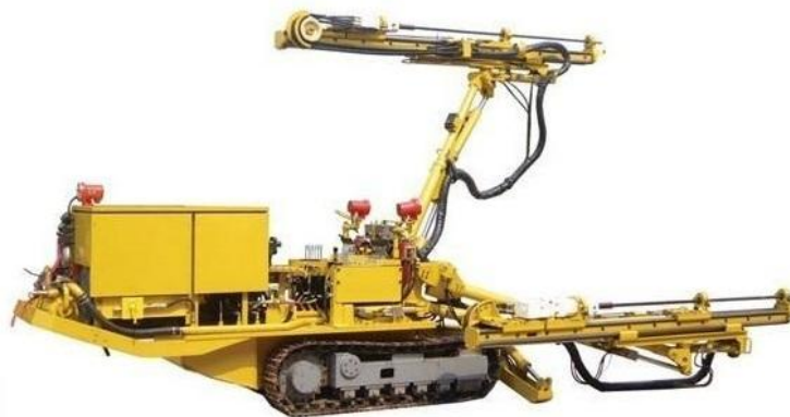
Figure 10 -Hydraulic Driver Crawler Drilling Rig 29
