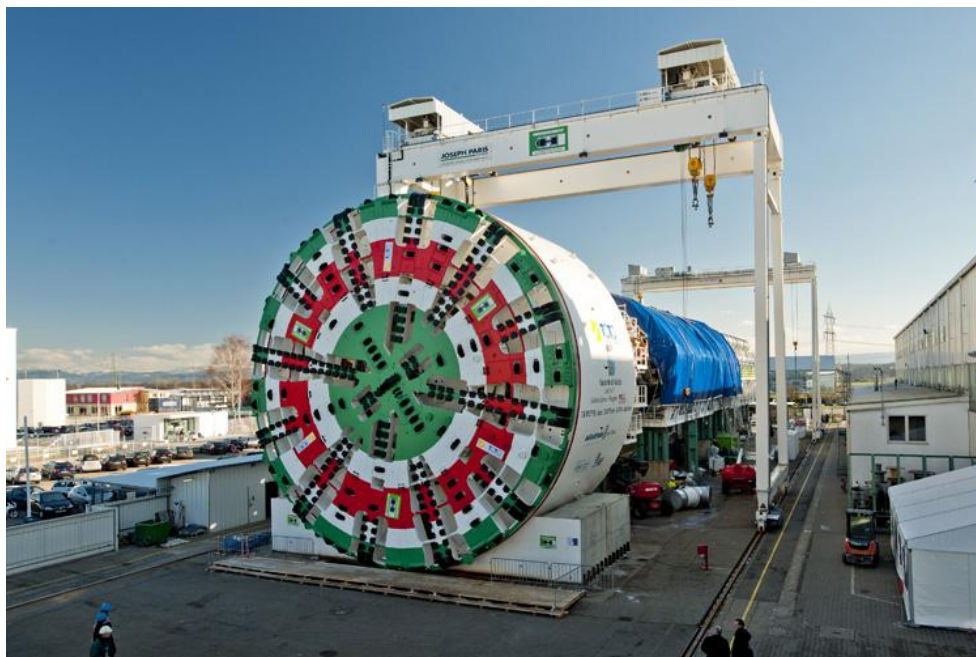
Figure 17 The Herrenknecht S-574 Earth Pressure Balance Shield 45
