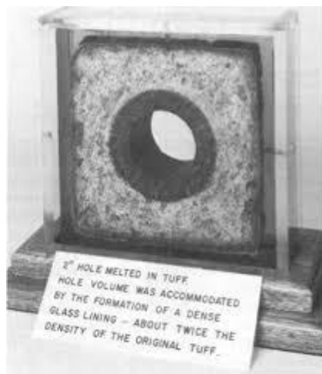
Figure 55 Typical glass-lined hole: Cross section of glass-lined hole (51-mm-diameter) melted in tuff rock 150
