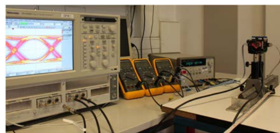
Figure 10. Photograph of receiver measurement set-up.
