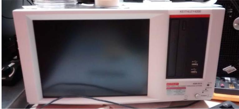
Figure 2.11.: Front view of the Keithley Parameter Analyser 4200
