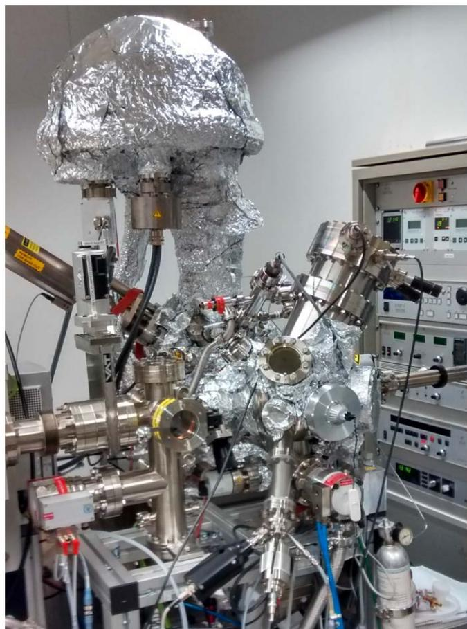
**Figure 2.12.:** The XPS setup used in this work
