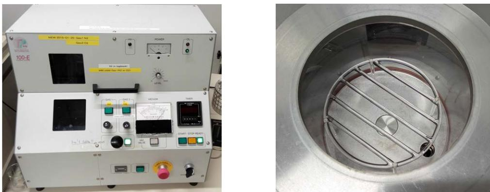
**Figure 2.4.:** The TePla plasma oxidation device, the right image shows the sample pedestal
