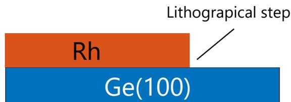
**Figure 3.14.:** A schematical drawing of the lithographically patterned step/edge of the Rh layer on Ge measured by AFM
