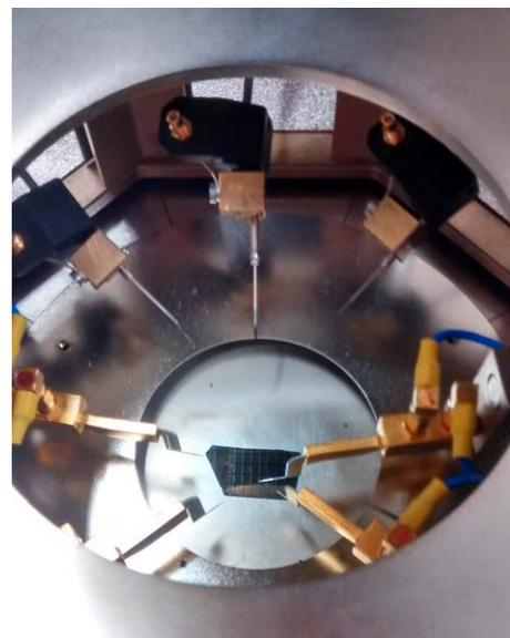
(b) View of the needles of the probe station in contact with a DUT
