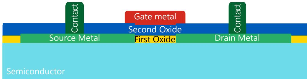
**Figure 2.8.:** Schematic of a SB-MOSFET with bilayer side
