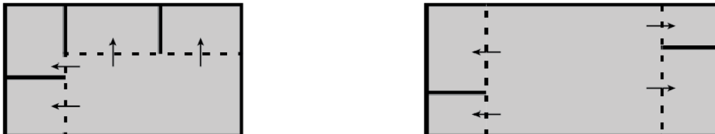
Fig. 67: Suggestions for core space, which gives access to other rooms and minimizes the transition area.
