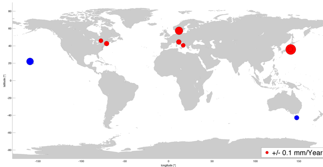
Figure 5.4: ZWD trends of the seasonal fit for GPS data, Red=Increase, Blue=Decrease, Trend = -0.3 to 0.8 mm/year
