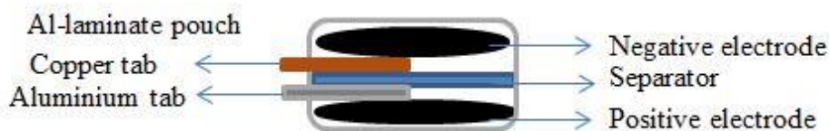
Figure 17. A cross sectional view of pouch cell configuration
