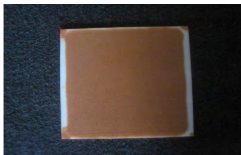
Figure 3.7: Thick film sample obtained by screen printing thick film paste PSB-1.5 on alumina substrate after sintering.
