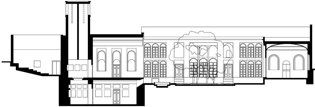
Figure 98, Tehrani house, section through central courtyard and wind catcher, source (Haji-Qassemi, Harirchi and Qelichkhani 2005, 191)
