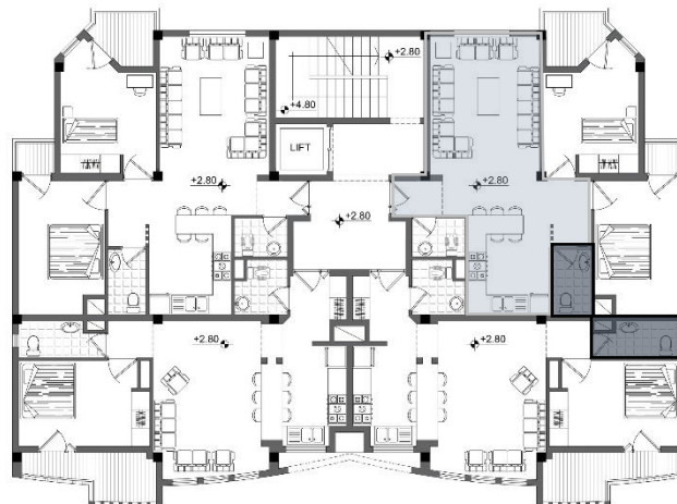
Figure 173, Sima Gostar case study unit and noisy spaces from neighboring units in the same floor
