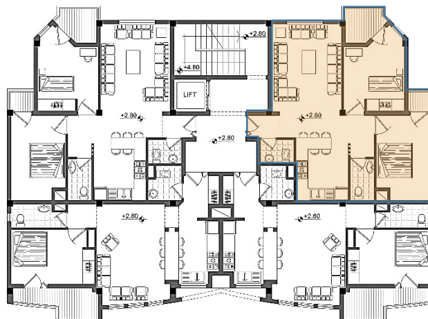
Figure 108, Sima Gostar typical floor plan and the selected unit as the case study among the four residential units in each floor, source (Honar Saraye Memari Consulting Engineers 2013)
