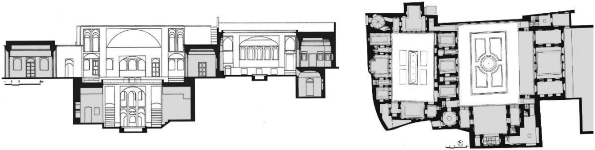
Figure 81, plan and section of Oloumi house with two level courtyard, Section and plan differ on scale, source: (Haji-Qassemi, Harirchi and Qelichkhani 2005, 104-111)
