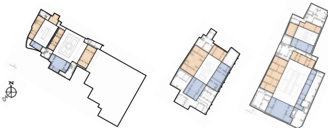
Figure 85, Left to right: plans of Oloumi, Tehrani and Lari houses in Yazd, with their due Southwest orientation, central courtyards and location of winter and summer spaces around the central courtyard, drawing by author
