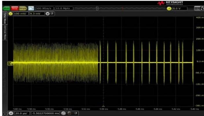
Figure 2.3: SHR followed by PHR – change of modulation format (measured on the output of an EVB1000, see section 2.2)
