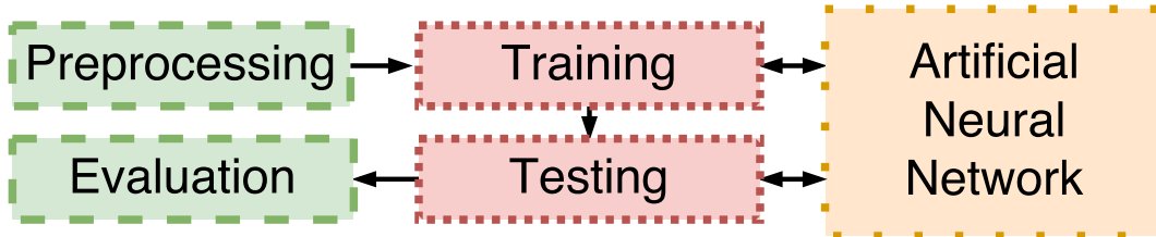
Figure 4.3: Hardware/software mapping, preprocessing and evaluation are performed on a X86 platform, training and testing of the neural network are controlled by processing system, neural network itself is implemented on programmable logic
