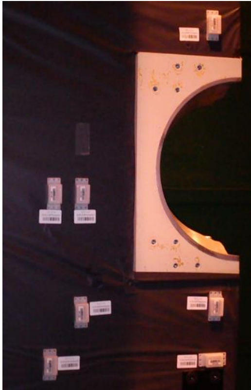
Figure 60: Photo of the central area of the HCAL detector front plane, showing part of the layout of the positions of the passive dosimeter boxes. None of the dosimeters cover the most exposed areas touching the central beam plug (white), necessitating the use of simulations for extrapolating the actual maximum dose that these modules are exposed to.
