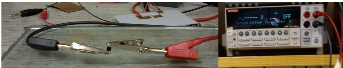
Figure 88: Close-up of the PiN-diode during measurement, which is held between two conductive clamps (left side) that are connected to the readout equipment (right side). The temperature sensor was located next to the Keithley power supply, about 40 cm away from the diode.
