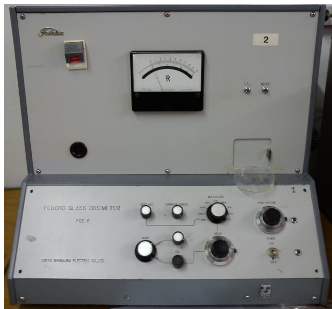
Figure 51: RPL readout equipment used by the CERN contractor in 2011.
