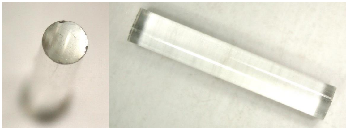
Figure 56: Two photos of the RPL sensor in passive box number 4IRCERPW0000016. Although small abrasions can be observed at the edges of the cylindrical crystal, the overall smoothness of the surface suggests a rather reliable outcome of the measurement. The difference to the Alanine sensor in the same passive box lies at around 12%.
