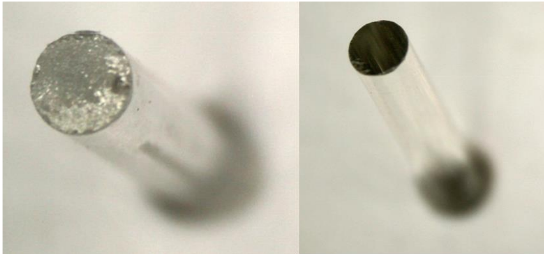
Figure 14: Comparison of the top surface of a damaged crystal (left) versus an intact crystal with a smooth surface (right). Dents and cracks like these influence the readout of the crystals through reflection and dispersion mechanisms that cannot be adjusted for. More varieties of damage can be found on other RPL dosimeters from this measurement campaign.
