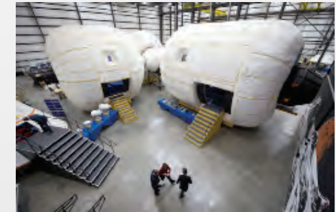
Abb.106: Full-scale model of the BA 330 inflatable space habitat, as seen at Bigelow Aerospace's Las Vegas facilities
