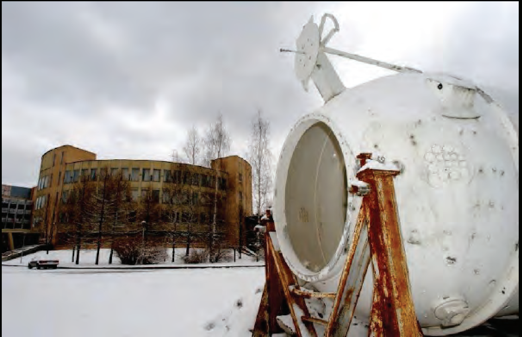
Abb. 194: This disused component was part of the training equipment used for cosmonauts who flew to the Mir station. It would be submerged in a giant pool, and the cosmonauts would practice spacewalking around it, avoiding the rocket thrusters and the antennae.
