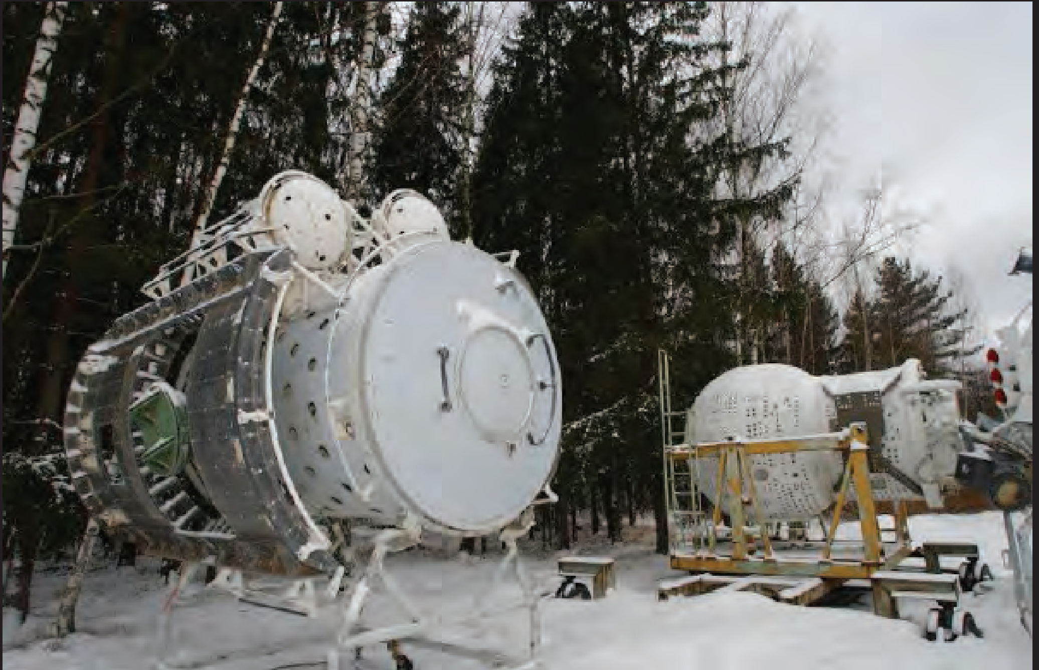
Abb.193: These components can be used during hydrolab EVA training to simulate the presence of components of the space station. These pieces are no longer used because they model part of the Mir station, which was de-orbited in 2001.
