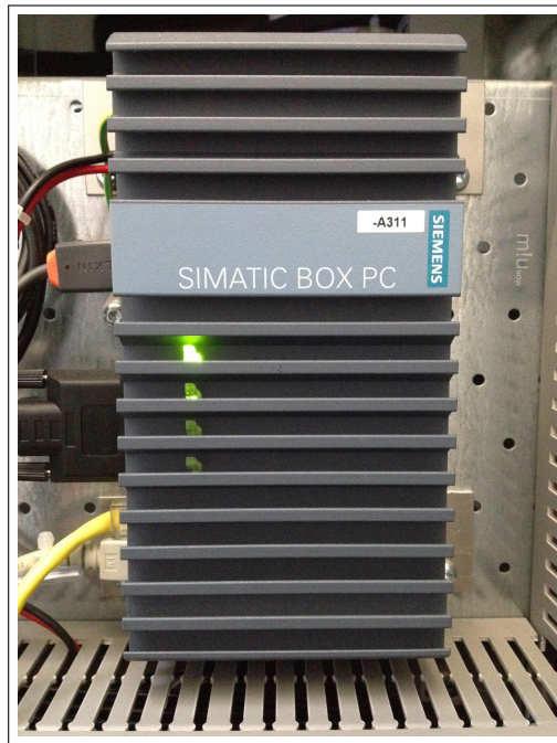
Figure 6.17: Target hardware for the control system: SIEMENS SIMATIC POX PC.
