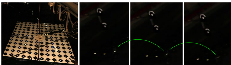
Figure 4.5: Left: the reference bar moved across the object space. Right: points moving away from the camera Line of Sight thus disappearing from the images.
