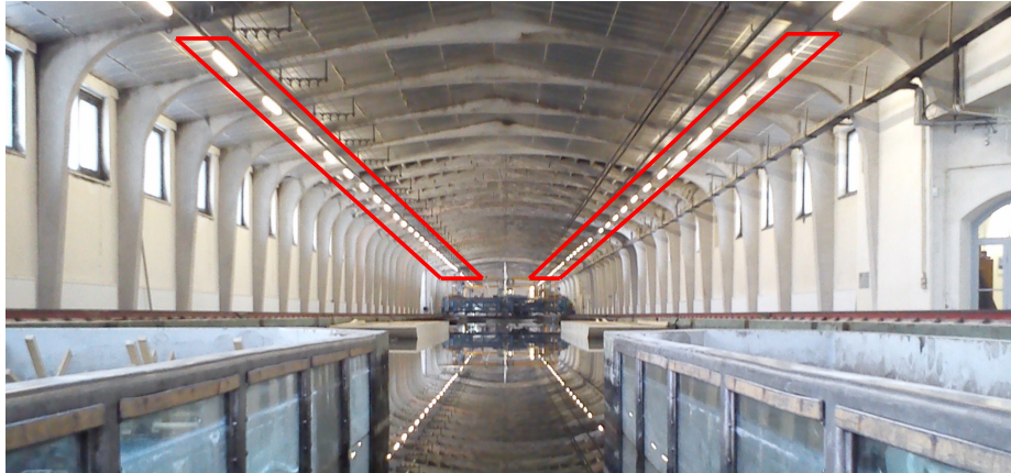
Figure 5.11: Two arrays of lamps are marked with red bounding boxes. The end points of the single lamps served as the control information.
