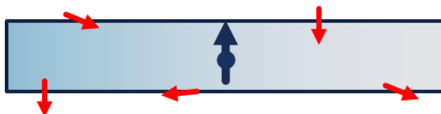
Figure 8 Schematic image of the implications of a flat, flake-like shape of the NDs with an assumed 111 texturation (with the NV - -center's main axis along the (111) crystal axis). The blue arrow marks the NV - -center while the red arrows represent external spins of interest (e.g. ROS).
